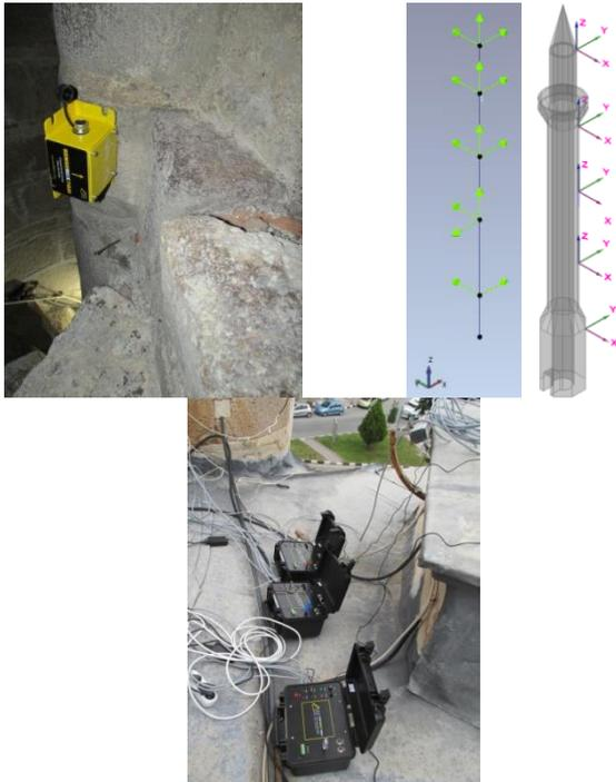
Fig. 7 Locations and directions of the accelerometers on the minaret and data acquisition system
