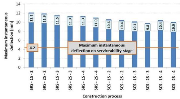
Fig. 7 Maximum instantaneous deflections of the 12 construction processes compared with those obtained in the structure's serviceability stage
