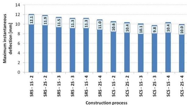
Fig. 5 Comparison of maximum short-term deflections of the 12 cases analysed
