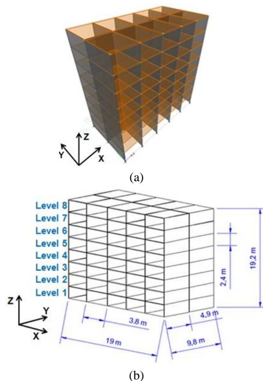
Fig. 1 The considered building: (a) Finite Elements Model, and (b) dimensions
