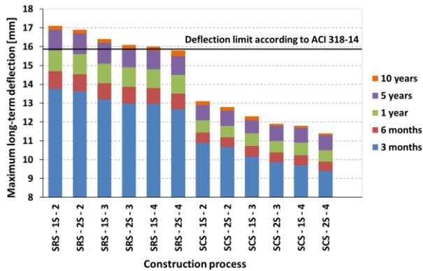
Fig. 8 Maximum long-term deflections of the 12 construction processes analyzed and the limit laid down by ACI 318-14
