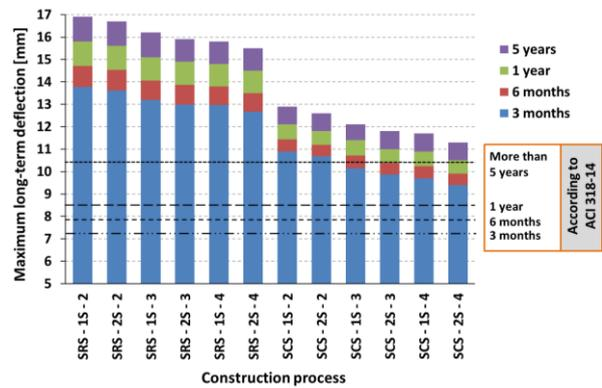
Fig. 9 Comparison of maximum long-term deflections of the 12 construction processes analyzed with those obtained by the simplified method in ACI 318-14
