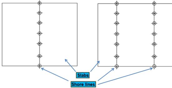
Fig. 3 Plan view of a slab with (a) a single line of shores and (b) double line of shores
