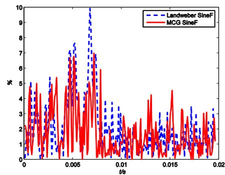
Fig. 13 The relative deviations for the identified sine force at noise level 5%
