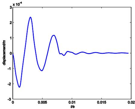
Fig. 9 The corresponding radial displacement response at Point 27
