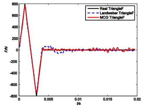
Fig. 12 The identified triangle force at noise level 5%; the number of iterations:  $N_{Landweber}=52$ ,  $N_{MCG}=16$
