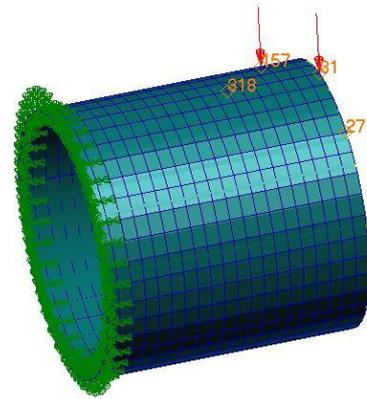
Fig. 8 The finite element model of thin-walled cylindrical shell
