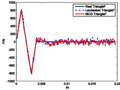
Fig. 5 The identified triangle force at noise level 5%; the number of iterations:  $N_{Landweber}=400$ ,  $N_{MCG}=42$
