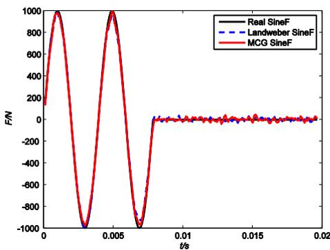
Fig. 11 The identified sine force at noise level 5%; the number of iterations:  $N_{Landweber}=52$ ,  $N_{MCG}=16$
