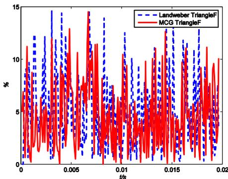
Fig. 7 The relative deviations for the identified triangle force at noise level 5%
