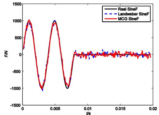
Fig. 4 The identified sine force at noise level 5%; the number of iterations:  $N_{Landweber}=400$ ,  $N_{MCG}=42$
