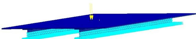
Fig. 1 The finite element model of stiffened plate
