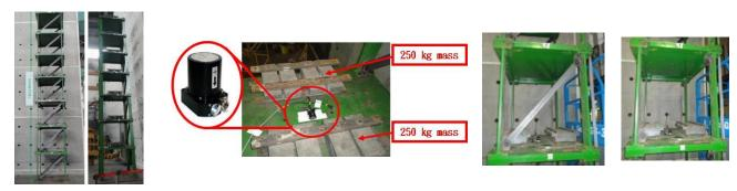
(a) Experimental specimen (b) Velocity meter and mass block of a single floor (c) braced Fig. 2 Layouts of experimental structure
