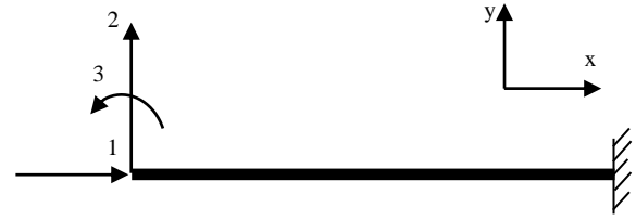
Fig. 4 A cantilever model for computing the relations between the nodal actions and basic deformation parameters
