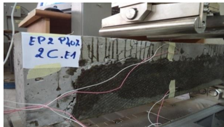
(a) Repaired by two plies
