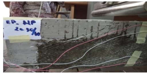
(b) Beam reinforced by two plies
