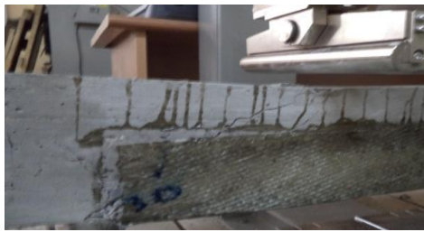
(a) Beam reinforced by one ply
