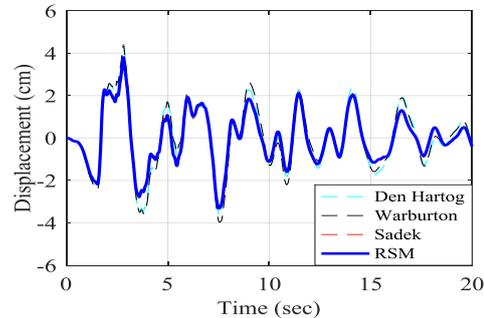
(f) Displacement with conventional and optimal TMD under Northridge earthquake
