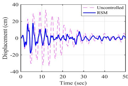
(a) Displacement with/without optimal TMD under El Centro earthquake
