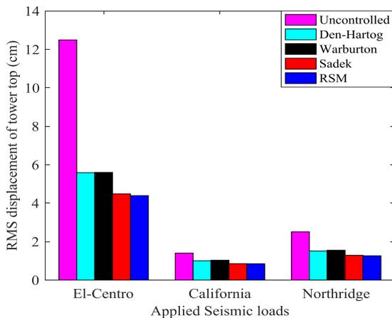
Fig. 11 Seismic response in terms of root mean square displacement of OWT structure
