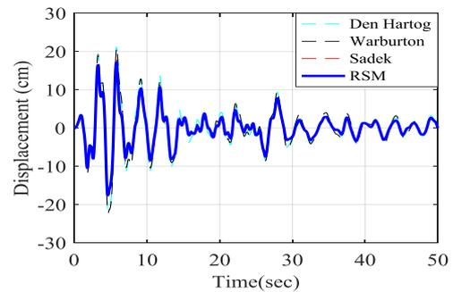
(b) Displacement with conventional and optimal TMD under El Centro earthquake
