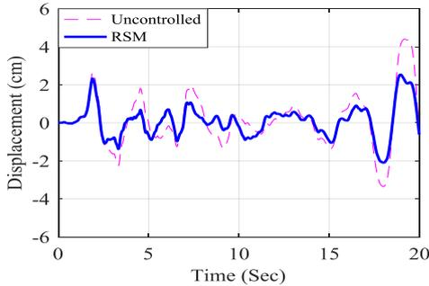
(c) Displacement with/without optimal TMD under California earthquake
