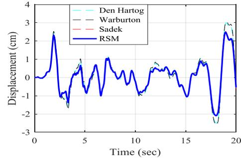
(d) Displacement with conventional and optimal TMD under California earthquake
