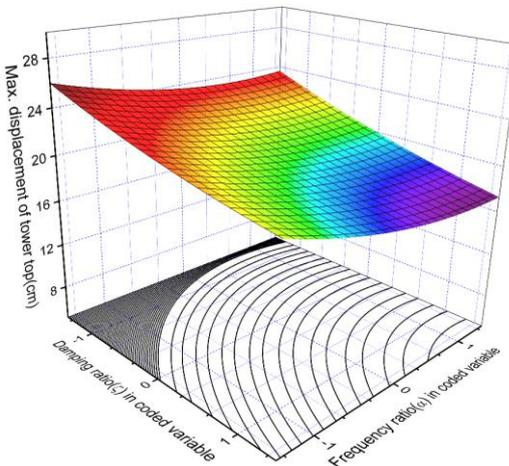
(b) 3D response surface and contour plot of tower top displacement ( $D_{tt}$ )
