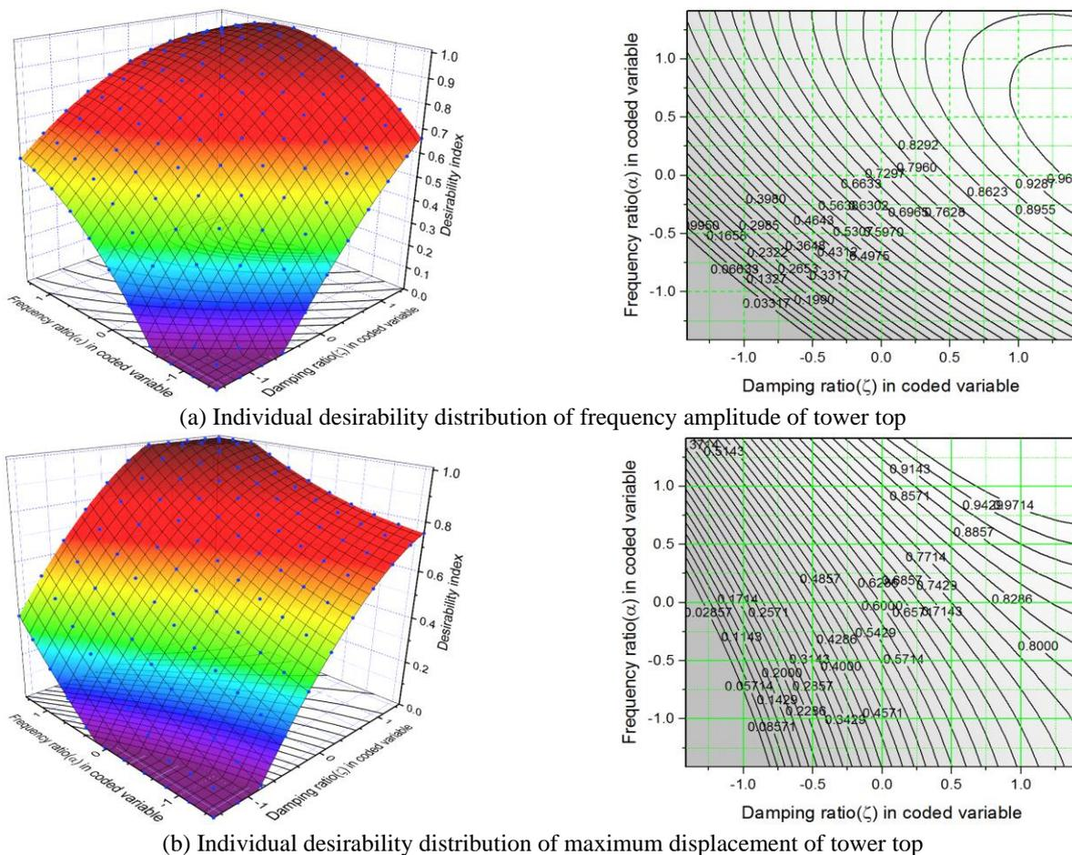
Fig. 7 Desirability distribution of individual response
