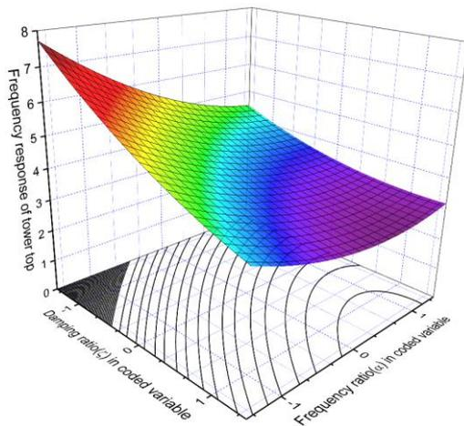
(a) 3D response surface and contour plot of frequency response of tower top ( $dB_{tt}$ )
