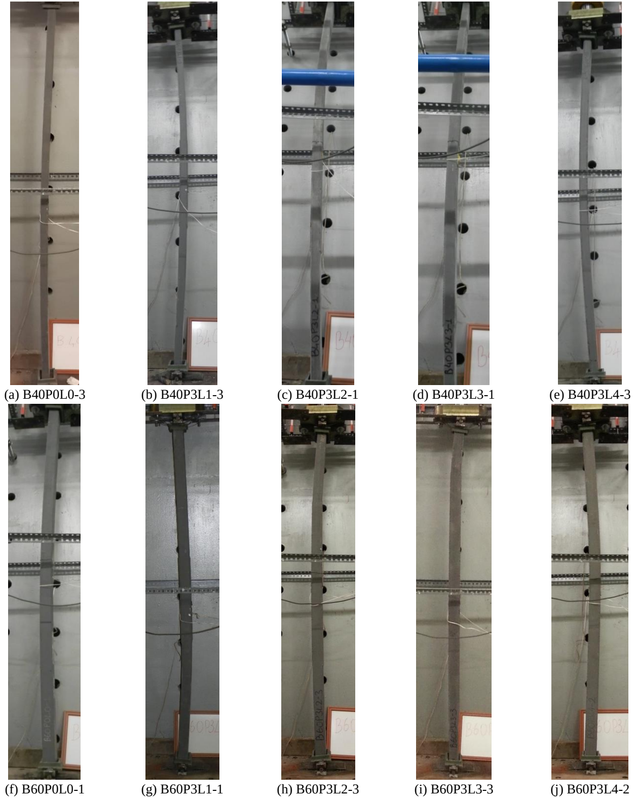
Fig. 11 Typical buckled shapes of slender test specimens
