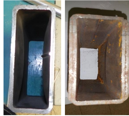
Fig. 10 Local buckling of larger side walls in SC specimens
