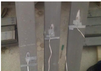
Fig. 5 Strain gages attached to the outermost fibers at the central cross section
