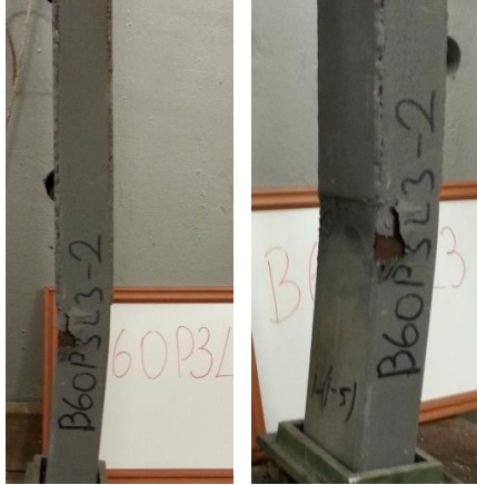
(b) Local buckling at the end of the reinforced region
