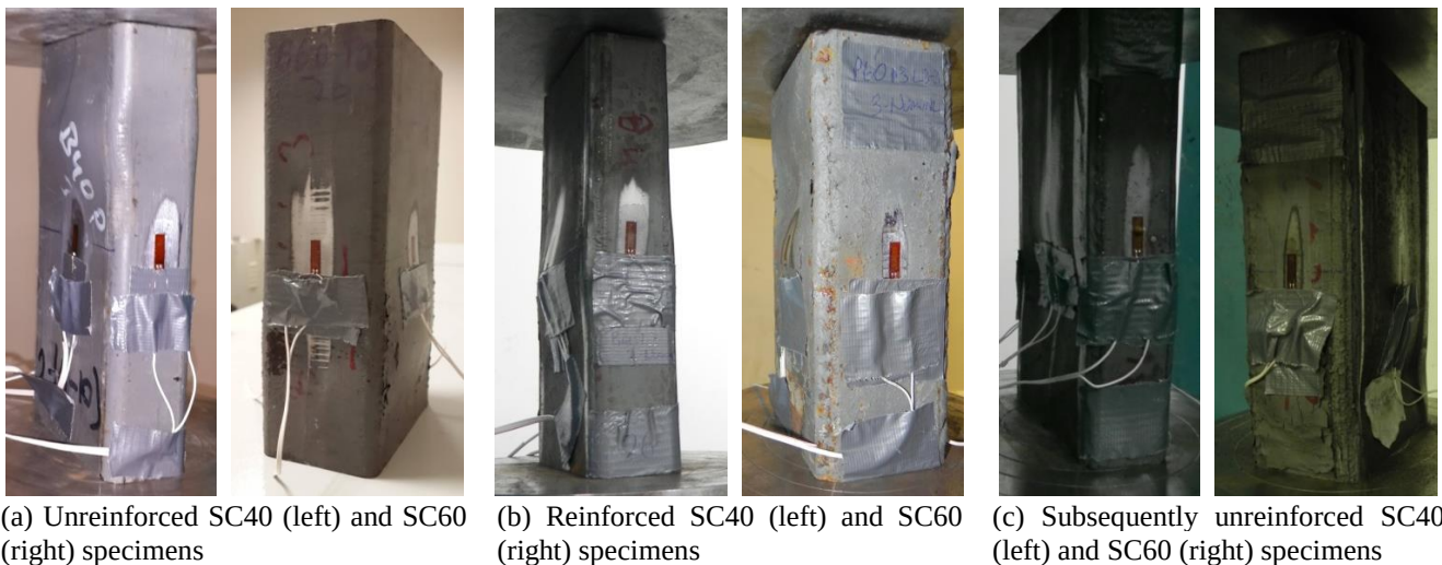
Fig. 7 Failure of stub-column specimens due to excessive local buckling
