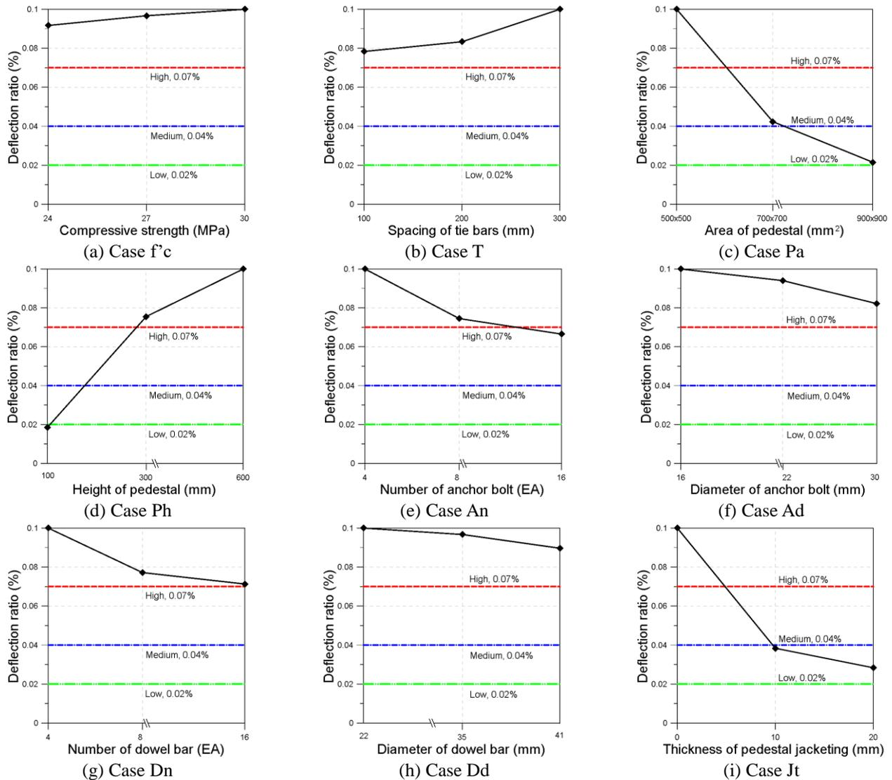
Fig. 8 Maximum deflection ratio of the pedestal with various reinforcement schemes at impact velocity of 30 km/h
