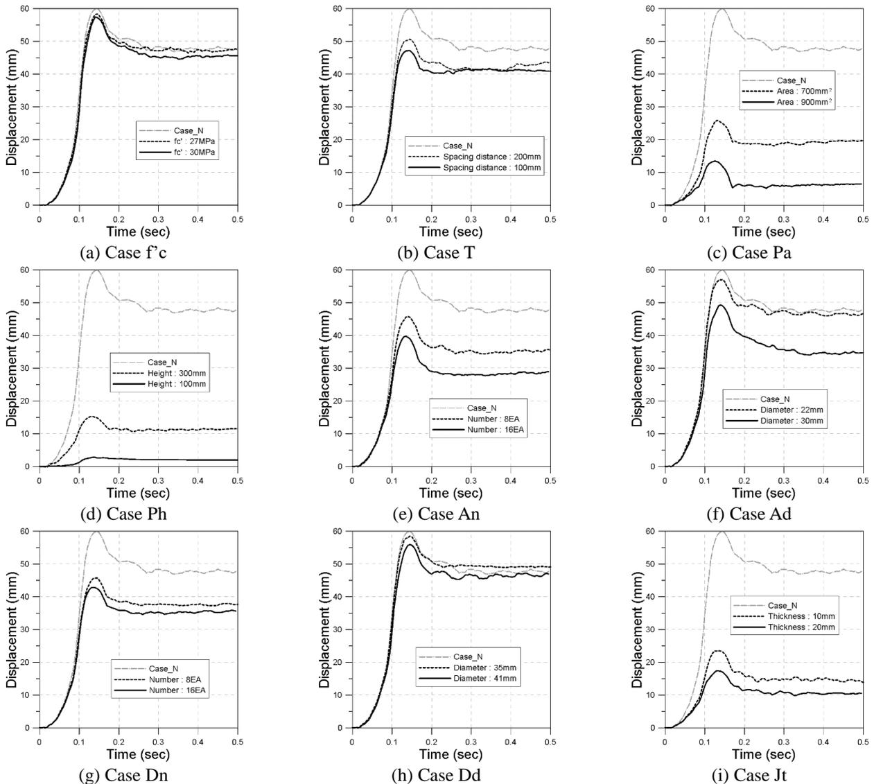
Fig. 7 Time history of horizontal displacement (Impact velocity=30km/h)
