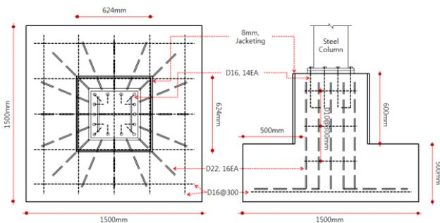
Fig. 14 Recommended detail of the reinforced footing pedestal (Case Ph + An + Dn + Jt)
