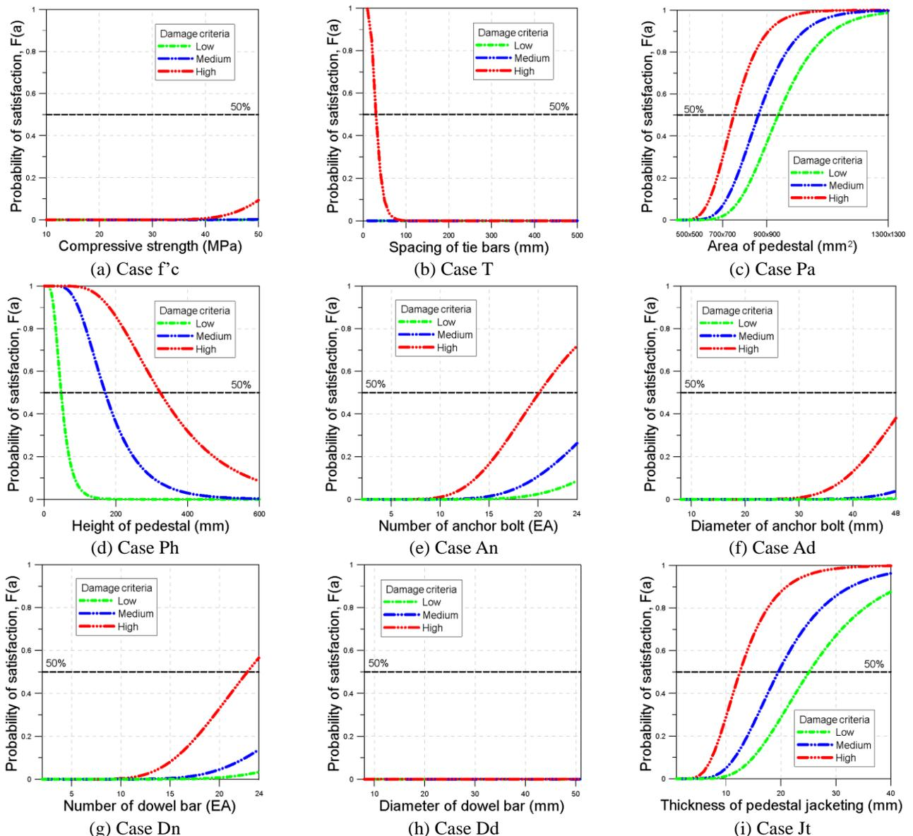
Fig. 11 Probability of satisfaction curve for various reinforcement methods at impact velocity of 30km/h
