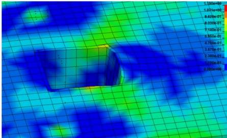
Fig. 6 Deformation and stress distribution of the column-pedestal and surrounding soil
