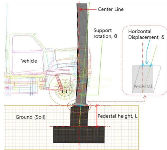
Fig. 4 Deformation of column-footing system subjected to vehicle collision
