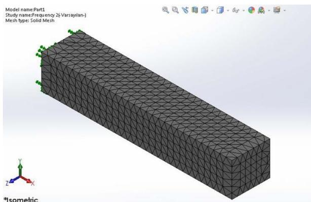
Fig. 10 Finite element model of FG beam after meshing
