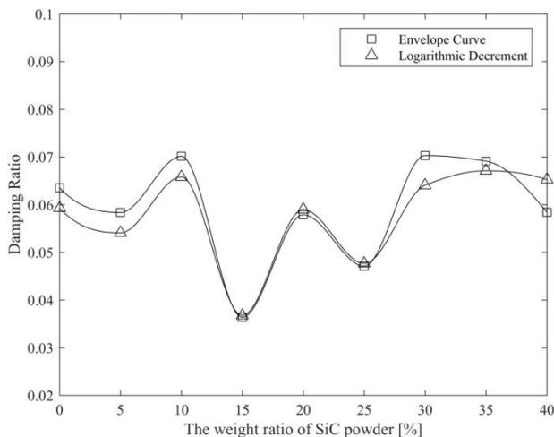
Fig. 15 Variation of damping ratio of the single layered beam (Model no:1)
