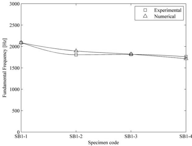
Fig. 13 Free vibration response of the multilayered sandwich beam (Model no:2)
