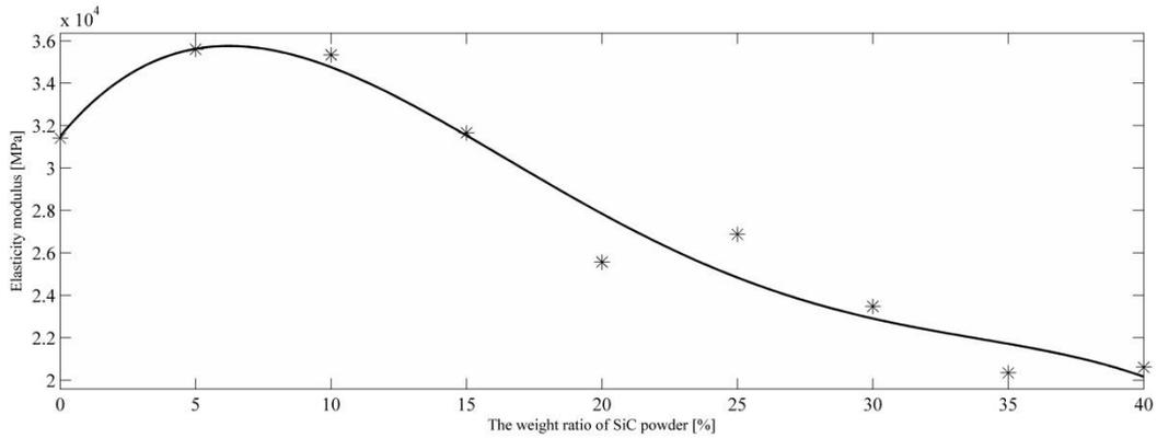
Fig. 6 Variation of the elasticity modulus with the weighting ratio of SiC powders
