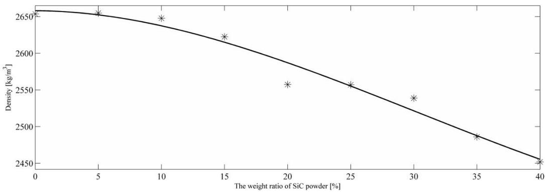
Fig. 7 Variation of the mass density with the weighting ratio of SiC powders
