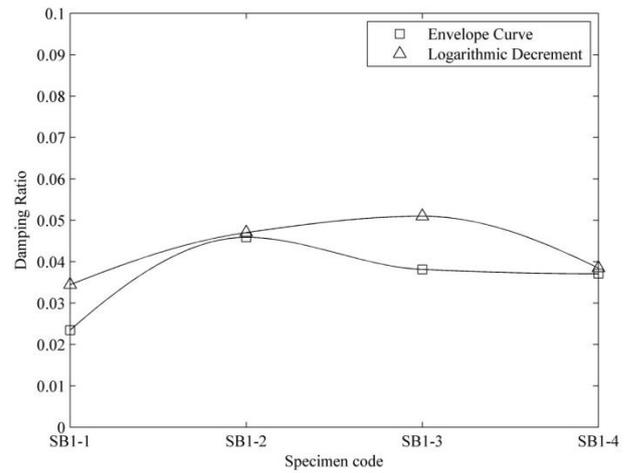
Fig. 16 Variation of damping ratio of the multilayered sandwich beam (Model no:2)
