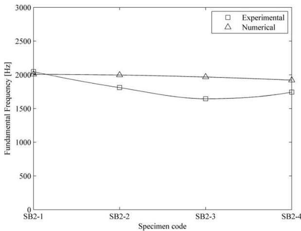
Fig. 14 Free vibration response of the multilayered sandwich beam (Model no:3)
