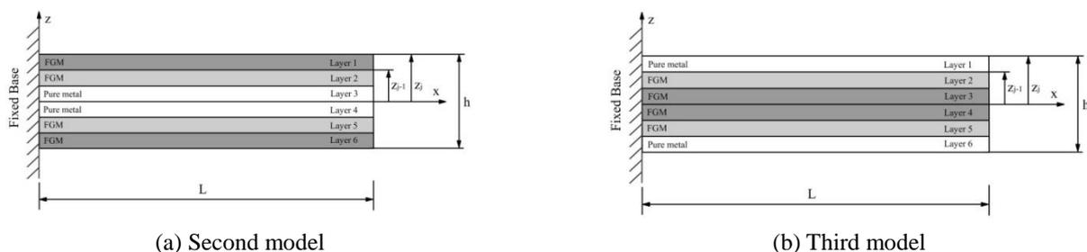
Fig. 1 Schematic representation of second and third models
