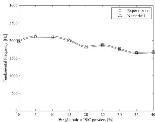
Fig. 12 Free vibration response of the single layered beam (Model no:1)
