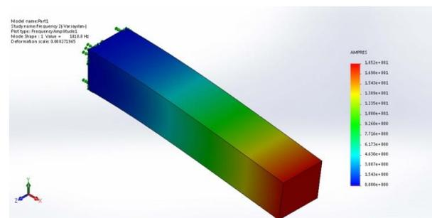
Fig. 11 Finite element model of FG beam after solution
