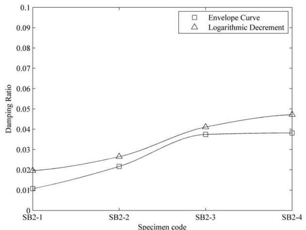
Fig. 17 Variation of damping ratio of the multilayered sandwich beam (Model no:3)
