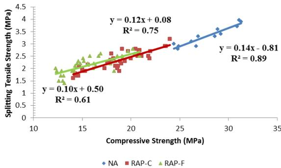
Fig. 10 Regression between splitting tensile strength and compressive strength for NA, coarse RAP, and fine RAP
