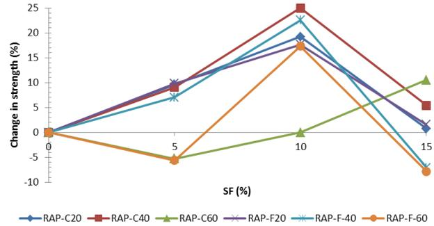
Fig. 9 Change in flexural strength with SF
