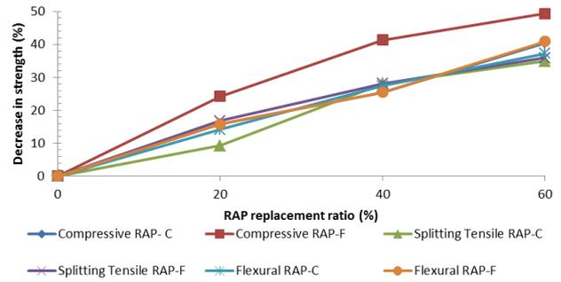
Fig. 4 Comparison of reduction rate in strength
