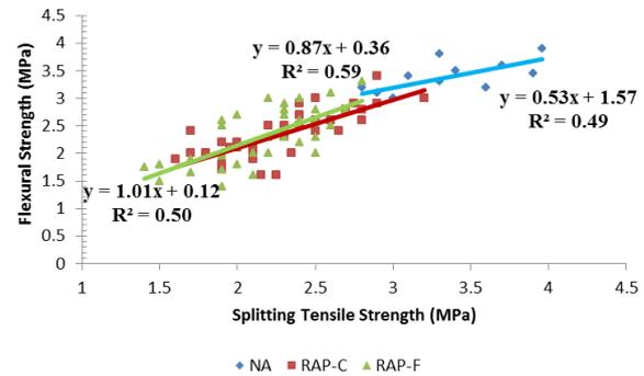
Fig. 11 Regression between flexural strength and splitting tensile strength for NA, coarse RAP, and fine RAP
