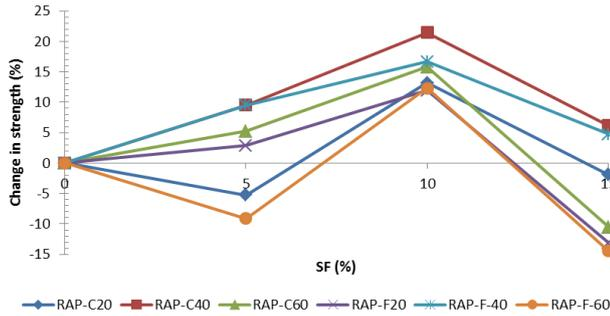
Fig. 7 Change in splitting tensile strength with SF
