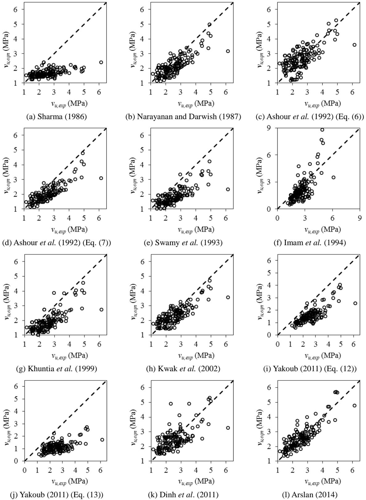
Fig. 5 The predictions by various equations vs. the experimental values
