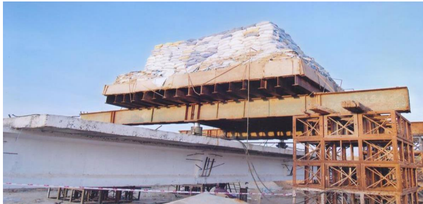
Fig. 3 Load test set up
