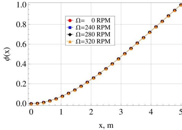
Fig. 7 The assumed mode shape  $\phi(x)$  for a non-uniform rotating Rayleigh cantilever, for different values of the uniform rotating speed  $\Omega$ , having an assumed fundamental frequency  $\omega = 140$  rad/s
