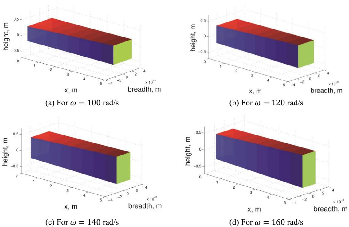
Fig. 3 Height and breadth variations for a Rayleigh cantilever beam, under an uniform axial load  $P = 500$  N, corresponding to the mass and stiffness variations shown in Fig. 2
