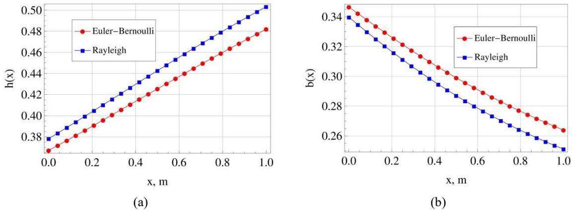
Fig. 12 Comparing the dimensions of a rectangular cross-section rotating cantilever Rayleigh and Euler-Bernoulli beam, for  $L = 1\text{m}$ ,  $\omega = 1000\text{ rad/s}$ ,  $\Omega = 2000\text{ RPM}$  and  $M_{tot} = 1000\text{ kg}$ : (a) Height variation, (b) breadth variation
