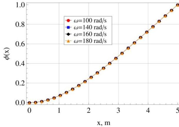
Fig. 4 The assumed mode shape  $\phi(x)$  for a non-uniform gravity-loaded Rayleigh cantilever, for different values of the assumed fundamental frequency  $\omega$
