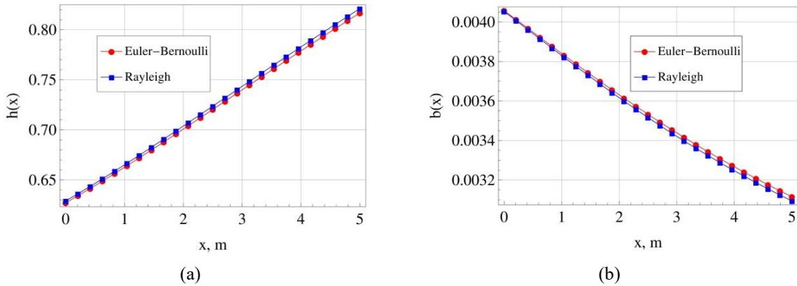
Fig. 11 Comparing the dimensions of a rectangular cross-section rotating cantilever Rayleigh and Euler-Bernoulli beam, for  $L = 5\text{m}$ ,  $\omega = 140\text{ rad/s}$ ,  $\Omega = 320\text{ RPM}$  and  $M_{tot} = 100\text{ kg}$ : (a) Height variation, (b) breadth variation
