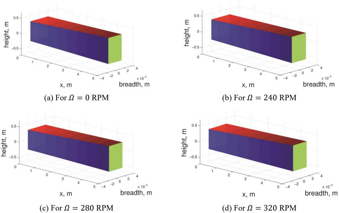
Fig. 9 Height and breadth variations for a rotating Rayleigh cantilever beam, corresponding to the mass and stiffness variations shown in Fig. 8
