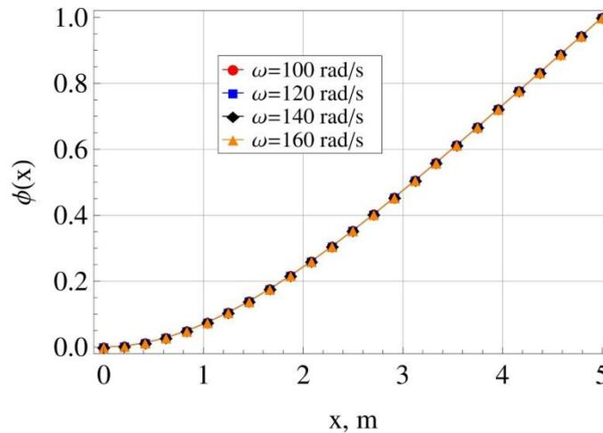
Fig. 1 The assumed mode shape  $\phi(x)$  for a non-uniform Rayleigh cantilever, under uniform axial load  $P = 500$  N, for different values of the assumed fundamental frequency  $\omega$
