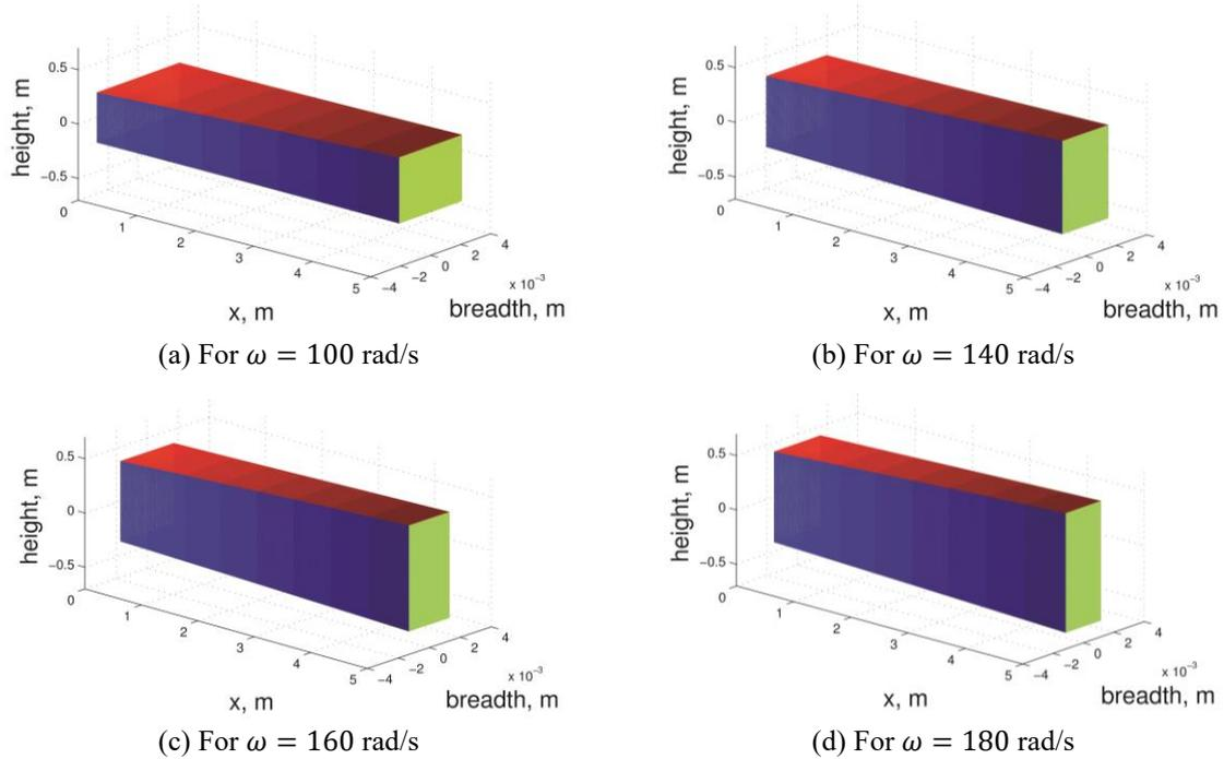
Fig. 6 Height and breadth variations for a gravity-loaded Rayleigh cantilever beam, corresponding to the mass and stiffness variations shown in Fig. 5
