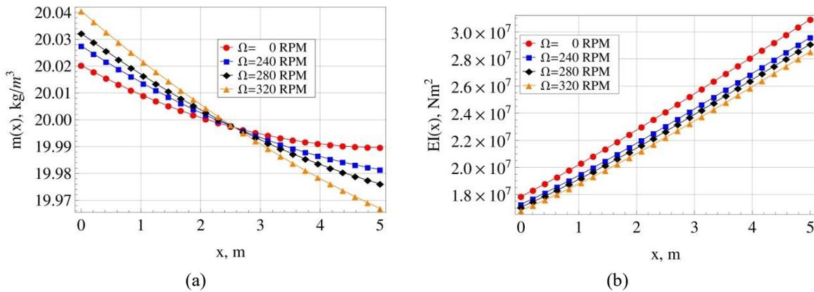
Fig. 8 Property variations for a non-uniform rotating Rayleigh cantilever, for different values of the uniform rotating speed  $\Omega$ , having an assumed fundamental frequency  $\omega = 140$  rad/s: (a) Mass variation, (b) stiffness variation
