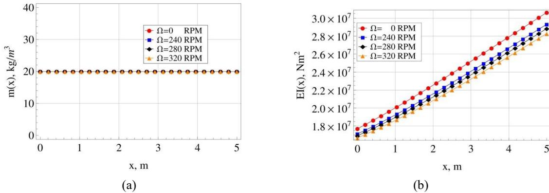
Fig. 10 Property variations for a non-uniform rotating Euler-Bernoulli cantilever beam, for different values of the uniform rotating speed  $\Omega$ , having an assumed fundamental frequency  $\omega = 140$  rad/s: (a) Mass variation, (b) stiffness variation
