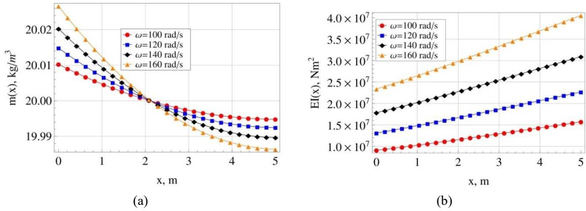
Fig. 2 Property variations for a non-uniform Rayleigh cantilever, under uniform axial load  $P = 500$  N, for different values of the assumed fundamental frequency  $\omega$ : (a) Mass variation, (b) stiffness variation
