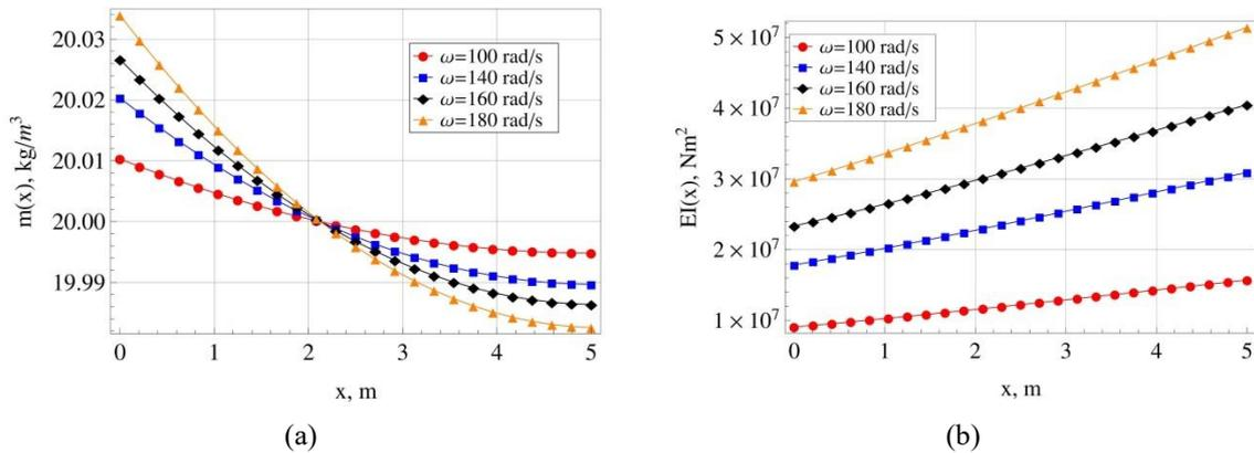
Fig. 5 Property variations for a non-uniform gravity-loaded Rayleigh cantilever, for different values of the assumed fundamental frequency  $\omega$ : (a) Mass variation, (b) stiffness variation
