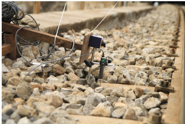
Fig. 6 LVDT sensor mounted on sleeper to monitor train movement
