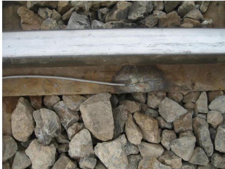
Fig. 7 Strain gauge mounted on rail heel to monitor train position during the tests
