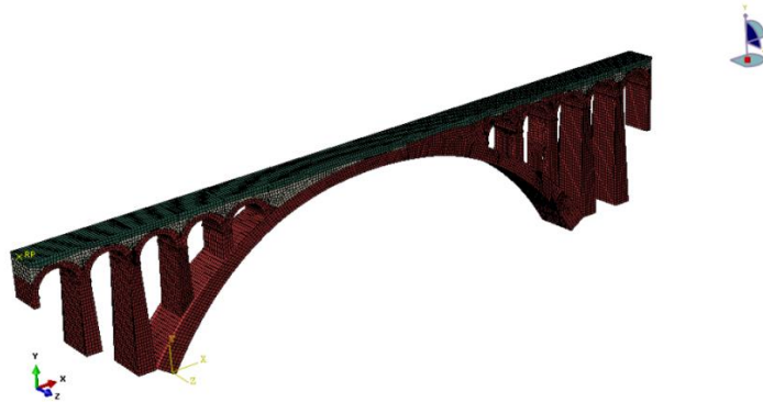
Fig. 14 3D F.E. model of Veresk in ABAQUES
