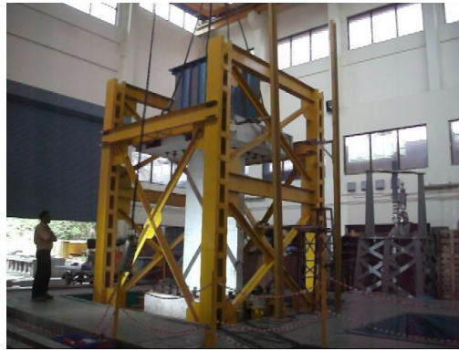
Fig. 8 Test setup (Shake table tests)
