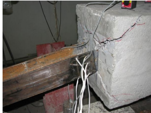
(f) Bending of pile (specimen 2)
