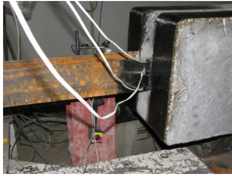
(a) Attaching of CFRP on the specimen 3
