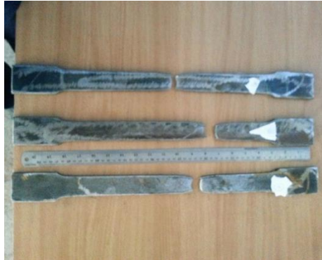
Fig. 8 Tensile test specimens of pile steels
