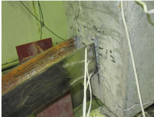
(e) Bending of pile (specimen 1)
