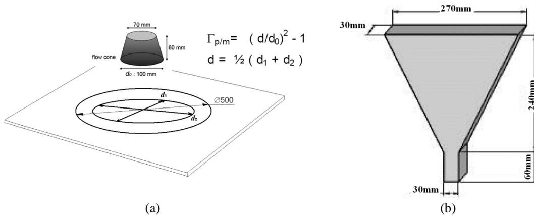
Fig. 3 (a) Flow test (b) V- funnel tests (EFNARC 2005)
