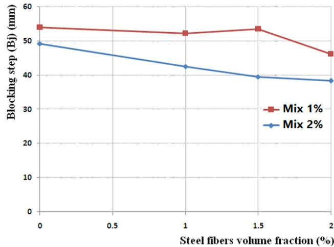
Fig. 13 Blocking step *BJ* in *J*-Ring tests
