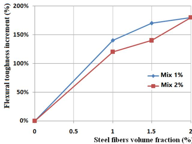
Fig. 25 Flexural toughness increment vs. different fibers volume fraction deflection
