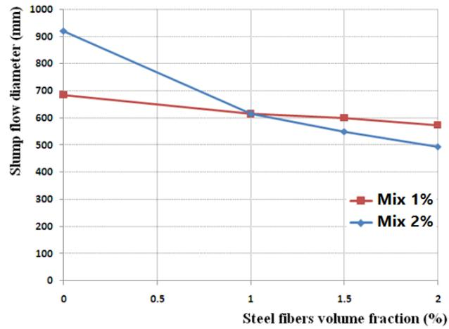
Fig. 8 Slump flow diameter
