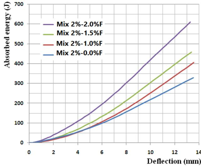
Fig. 24 Absorbed energy vs. deflection curves for Mix 2% beams
