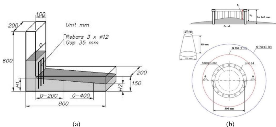
Fig. 4 (a) L-Box test (EFNARC 2005) (b) J ring test (Gencel *et al.* 2011)
