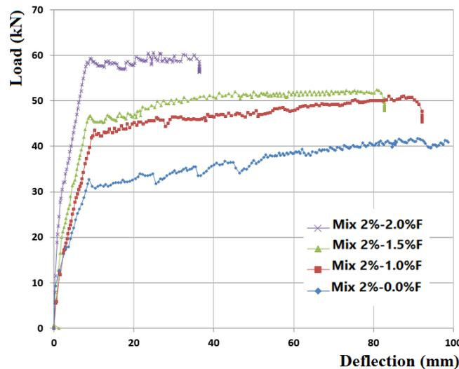
Fig. 17 Load-deflection curves from beams tests performed from Mix 2% with different ratio of steel fibers
