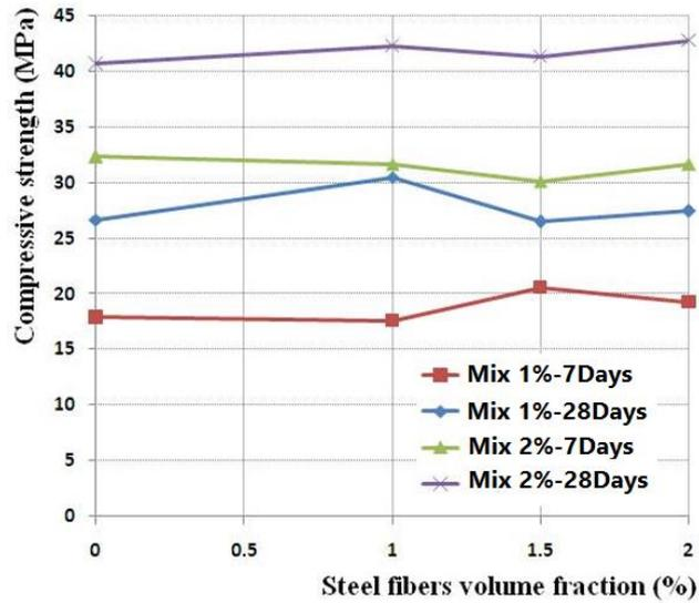
Fig. 14 Compressive strength results
