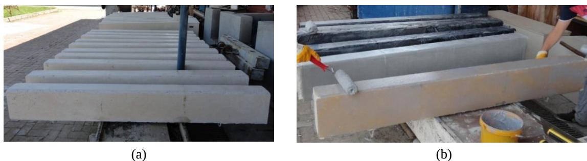
Fig. 2 (a) Drying and surface preparation of beam (b) Applying the epoxy resin to the beam surface (c) Bonding of glass fibers to beam surface (d) Bonding of carbon fiber to beam surface (e) Applying the epoxy resin to the beam surface (f) epoxy impregnation, (g) Bonding of carbon fiber to beam surface with the 45^\circ angle
