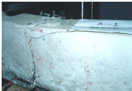
Fig. 5 Failure mode of the specimens of Group A
