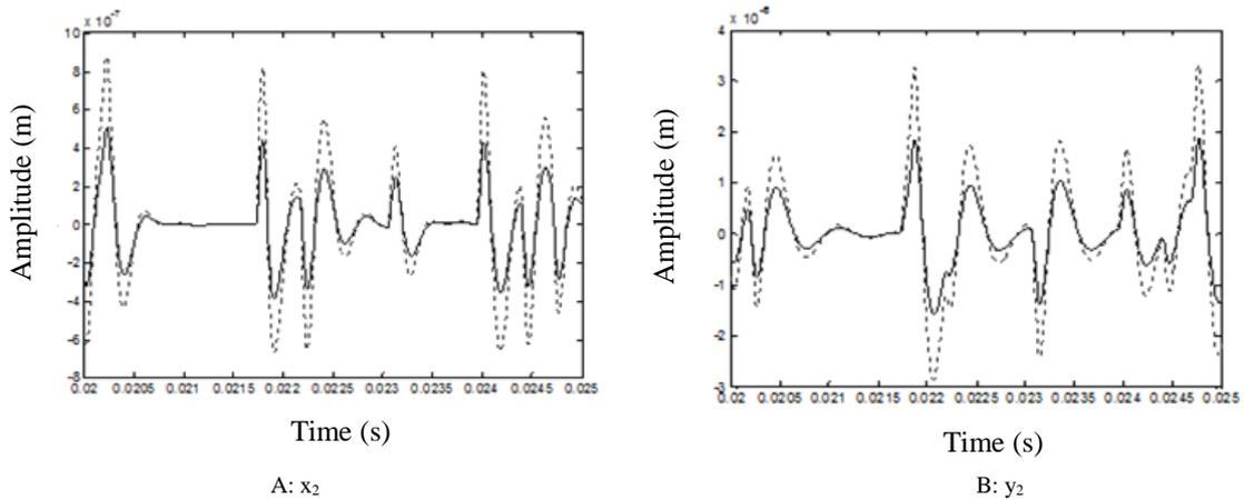
Fig. 5 Time dynamic response of the second bearing — without assembly defect; ..... with assembly defect ( $a=1 \text{ mm}$ )
