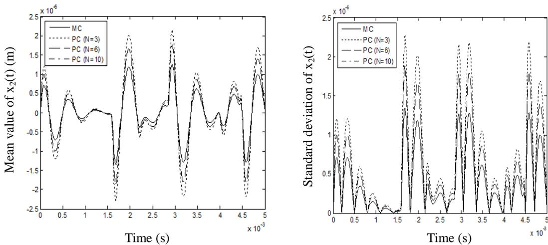
Fig. 13 Mean value and standard deviation of  $x_2(t)$  considering uncertain assembly defect  $\sigma_a = 15\%$
