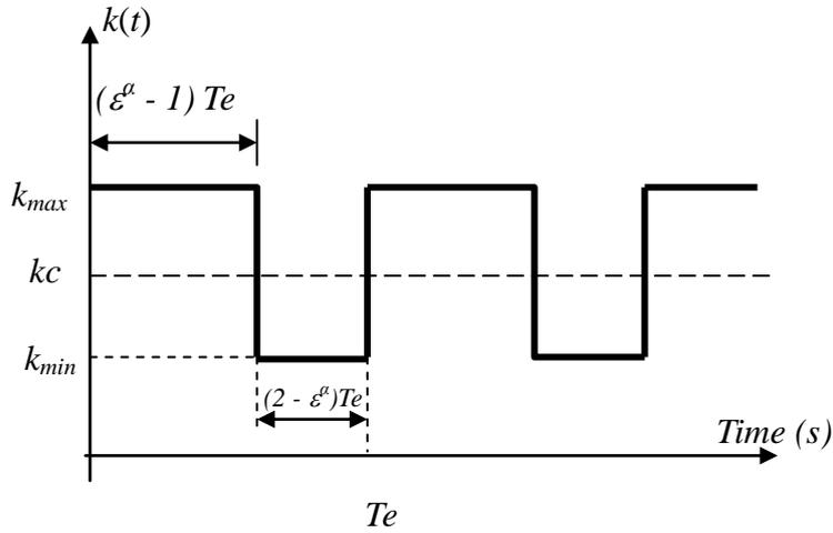
Fig. 2 Modelling of the mesh stiffness variation
