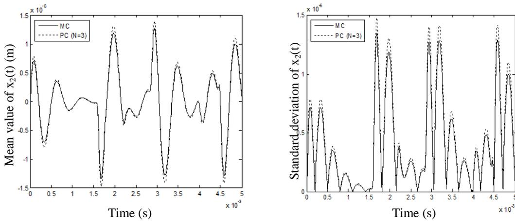
Fig. 11 Mean value and standard deviation of  $x_2(t)$  considering uncertain bearings stiffness  $\sigma_{k_x} = \sigma_{k_y} = 3\%$
