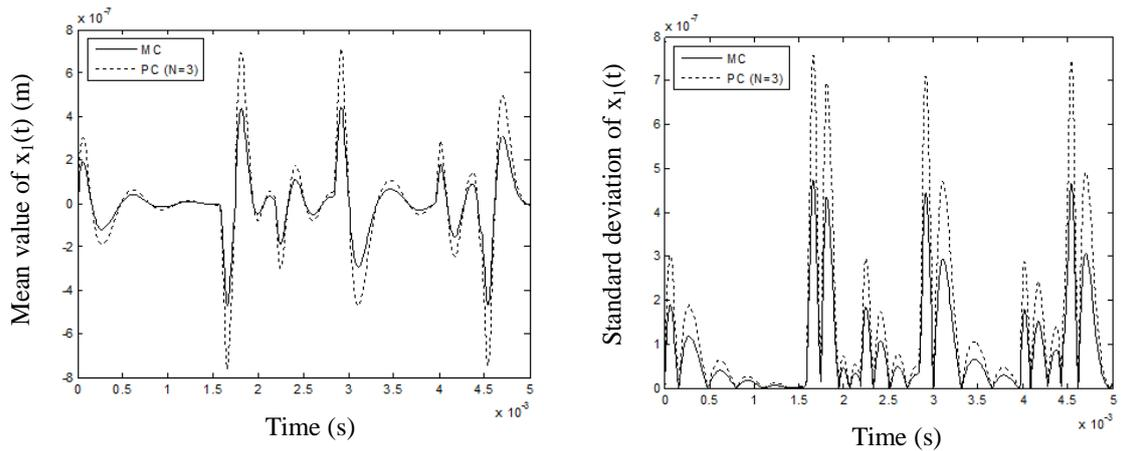
Fig. 8 Mean value and standard deviation of  $x_1(t)$  considering uncertain assembly defect  $\sigma_a=7\%$
