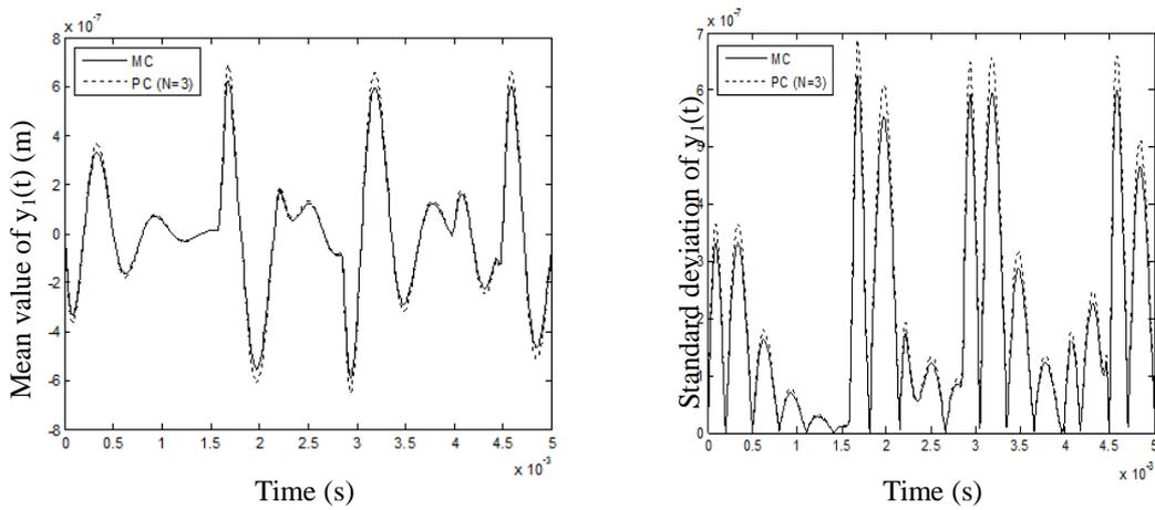
Fig. 10 Mean value and standard deviation of  $y_1(t)$  considering uncertain damping coefficients  $\sigma_{c_x} = \sigma_{c_y} = 7\%$
