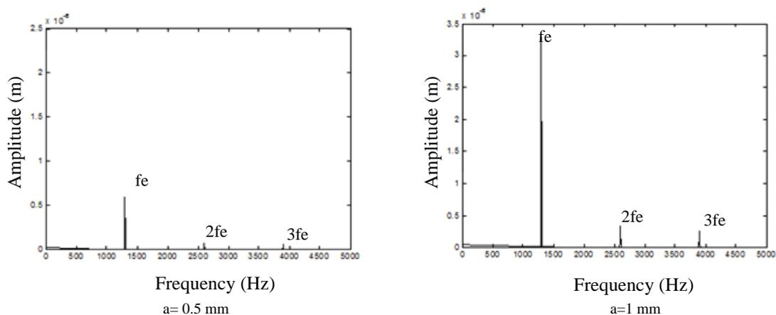
Fig. 6 Frequency responses of the first bearing with assembly defect
