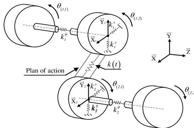
Fig. 1 Global dynamic model of the one stage gear system
