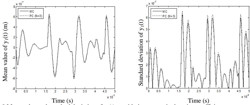
Fig. 9 Mean value and standard deviation of  $y_1(t)$  considering uncertain damping coefficients  $\sigma_{c_x} = \sigma_{c_y} = 3\%$
