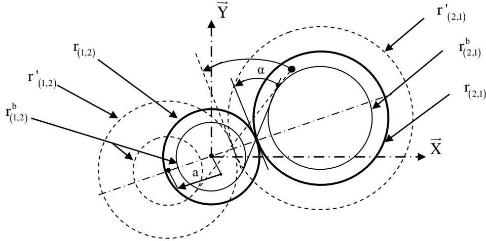
Fig. 3 Assembly defect
