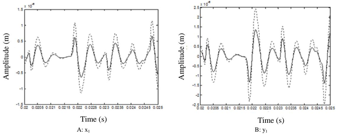
Fig. 4 Time dynamic response of the first bearing — without assembly defect; ..... with assembly defect ( $a=1 \text{ mm}$ )
