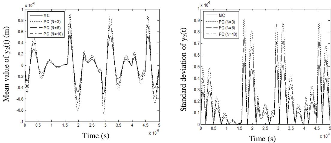
Fig. 14 Mean value and standard deviation of  $y_2(t)$  considering uncertain assembly defect  $\sigma_a=15\%$
