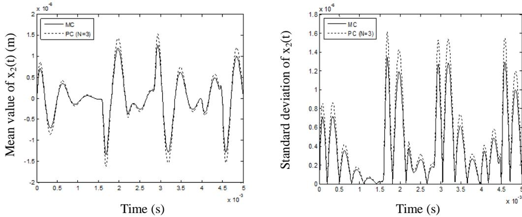
Fig. 12 Mean value and standard deviation of  $x_2(t)$  considering uncertain bearings stiffness  $\sigma_{k_x} = \sigma_{k_y} = 7\%$
