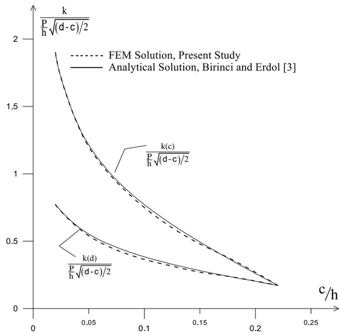
Fig. 12 Comparisons of analytical solution with FEM solution for the normalized stress-intensity factors with  $c/h$  for an internal crack ( $a/h = 2, h_1/h = 0.5, b/h = 1, \beta = 0.22$ )
