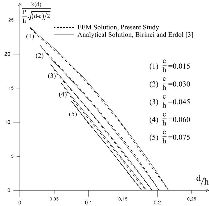
Fig. 11 Comparisons of analytical solution with FEM solution for the normalized stress-intensity factors  $k(d)$  with  $d/h$  for various values of  $c/h$  for the case of an internal crack ( $a/h = 1, h_1/h = 0.3, b/h = 1, \beta = 0.1$ )
