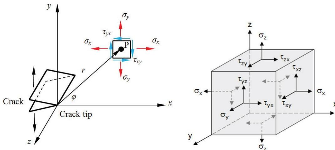
Fig. 3 Infinite plate with a central crack and the Cauchy stress tensor
