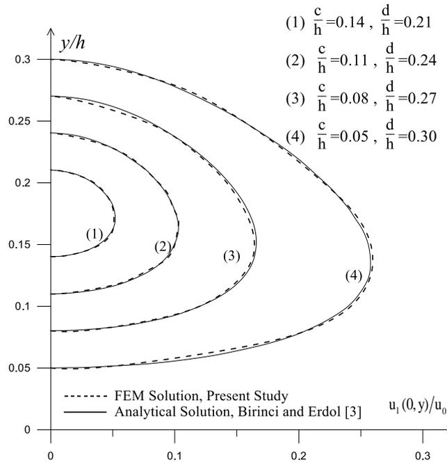
Fig. 15 Comparisons of analytical solution with FEM solution for the normalized crack surface displacement for various of  $c/h$  and  $d/h$  for the case of an internal crack ( $a/h = 0.1, h_1/h = 0.7, b/h = 1, \beta = 1$ )
