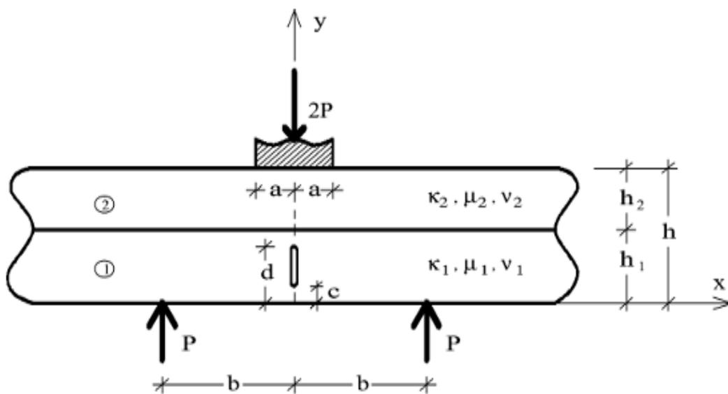
Fig. 1 Geometry of the layered composite containing a crack in its lower layer
