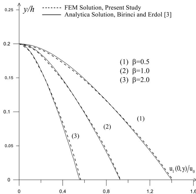
Fig. 16 Comparisons of analytical solution with FEM solution for the normalized crack surface displacement for various of  $\beta$  for the case of an internal crack ( $a/h = 0.05, h_1/h = 0.5, b/h = 1, d/h = 0.2$ )
