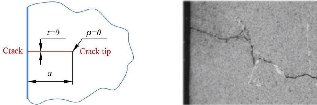
Fig. 2 Ideal computational model of a crack and the real crack in the material
