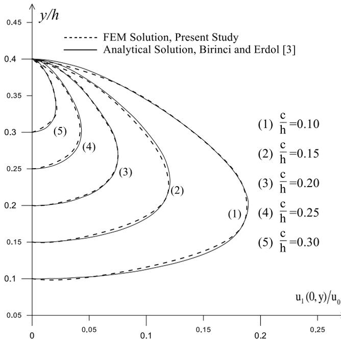
Fig. 14 Comparisons of analytical solution with FEM solution for the normalized crack surface displacement for various of  $c/h$  for the case of an internal crack ( $a/h = 0.15$ ,  $h_1/h = 0.8$ ,  $b/h = 1$ ,  $d/h = 0.4$ ,  $\beta = 0.1$ )
