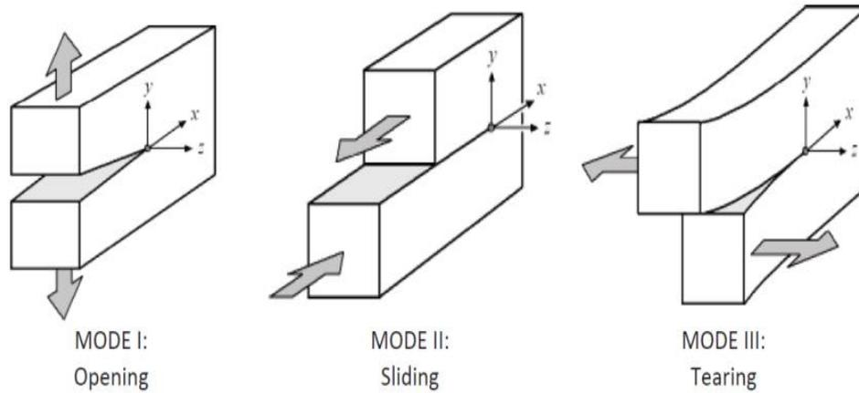
Fig. 4 Three modes of the crack deformation
