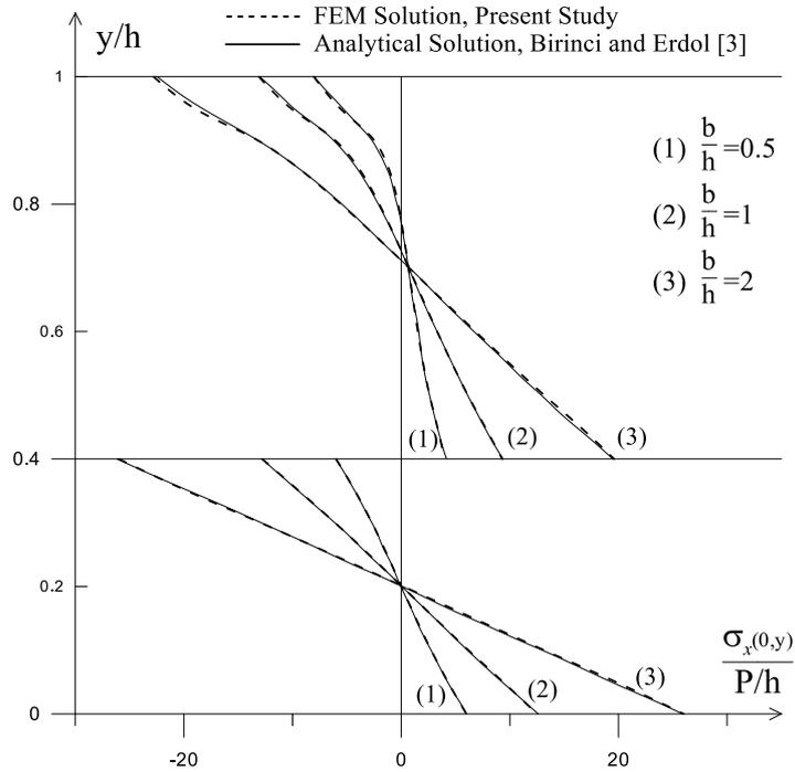
Fig. 9 Comparisons of analytical solution with FEM solution for the normalized axial stress  $\sigma_x(0, y)/(\frac{P}{h})$  in the layered composite without a crack for various values of  $b/h$  ( $a/h = 0.1, h_1/h = 0.4, \beta = 0.5$ )
