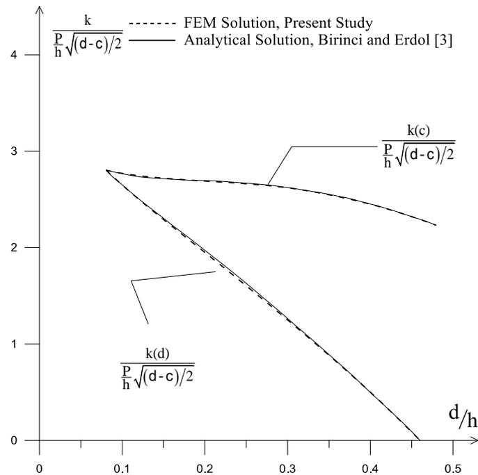
Fig. 10 Comparisons of analytical solution with FEM solution for the normalized stress-intensity factors with  $d/h$  for an internal crack ( $a/h = 1, h_1/h = 0.7, b/h = 1, c/h = 0.08, \beta = 0.1$ )
