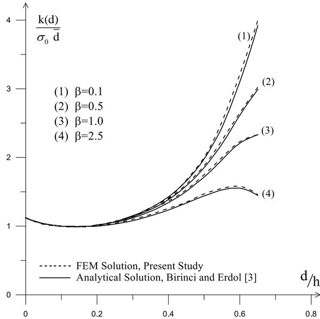
Fig. 13 Comparisons of analytical solution with FEM solution for the normalized stress-intensity factors  $k(d)$  with  $d/h$  for various values of  $\beta$  for the case of an edge crack ( $a/h = 0.2$ ,  $h_1/h = 0.8$ ,  $b/h = 1$ ,  $\sigma_0 = \sigma_{1x}^*(0,0)$ )
