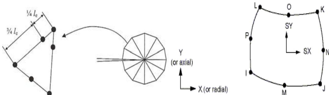
Fig. 7 Element 8-node PLANE 183
