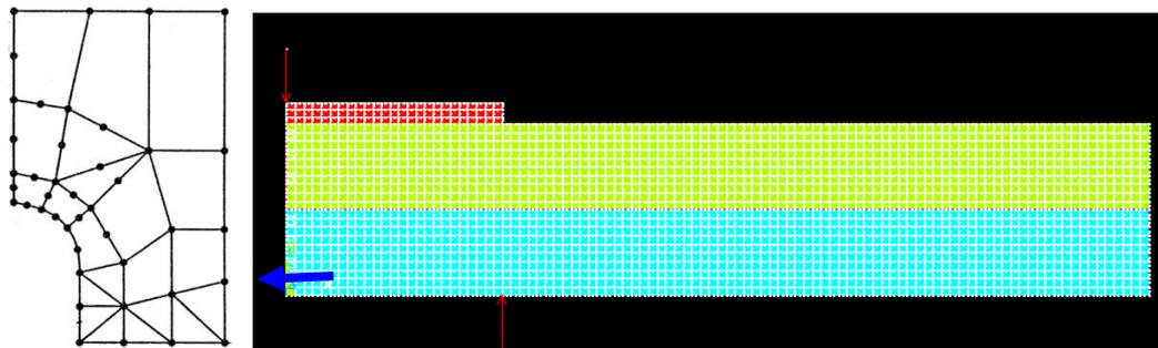
Fig. 6 An edge crack and the finite element mesh
