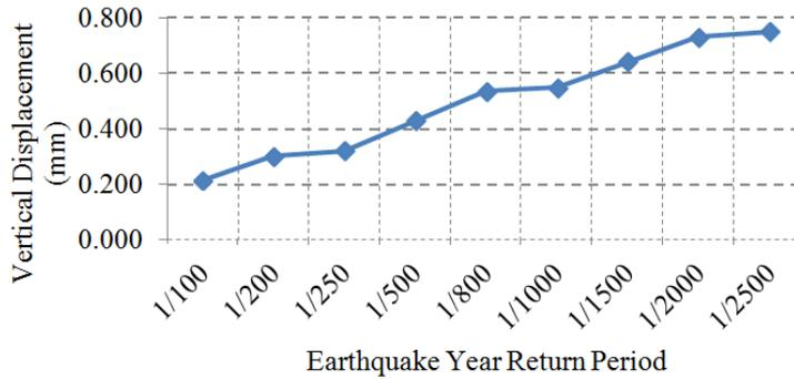
(b) Vertical displacement vs earthquake YRI
