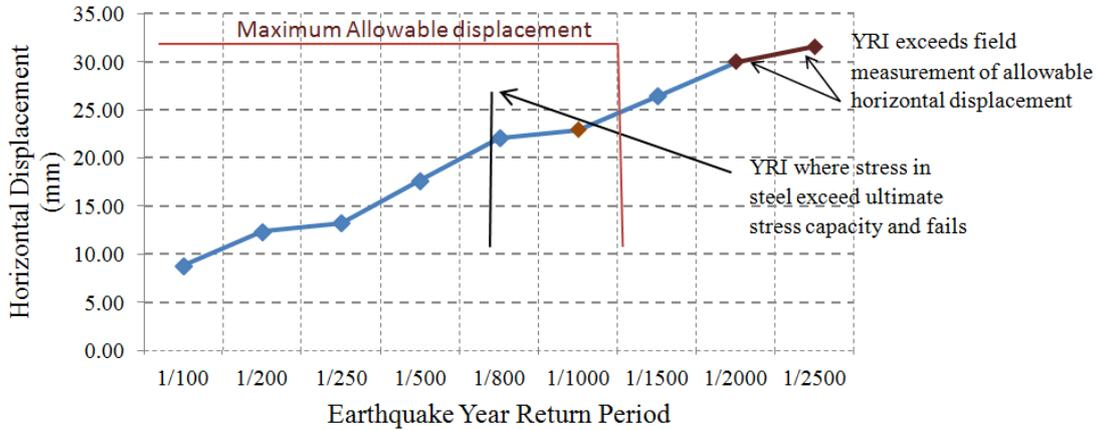
(a) Horizontal displacement vs earthquake YRI
