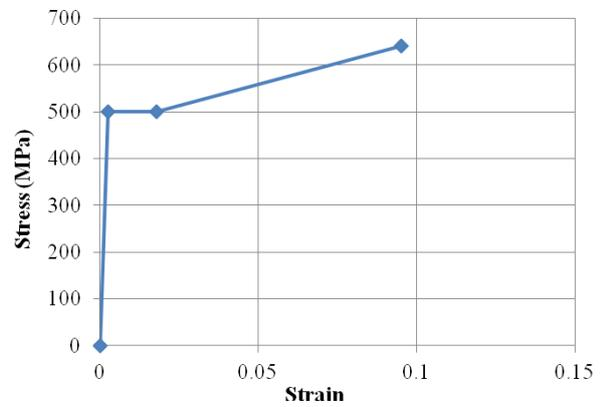
Fig. 4 Stress-strain relationship for steel reinforcement
