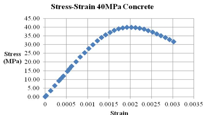
Fig. 5 40MPa concrete stress-strain diagram
