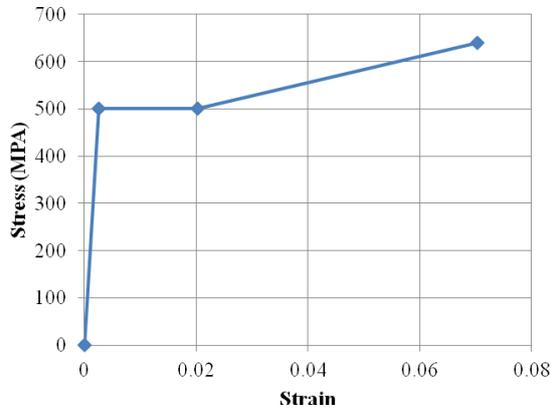
Fig. 3 Stress-strain relationship for steel truss
