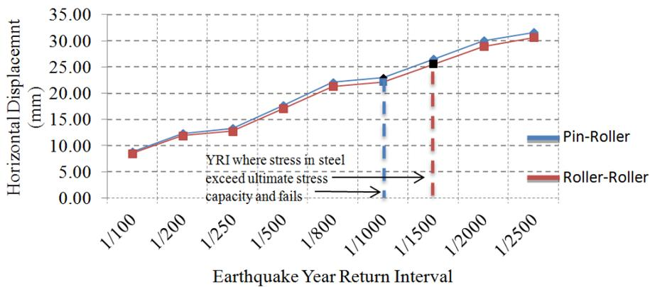
Fig. 10 Comparison of horizontal displacement design graph
