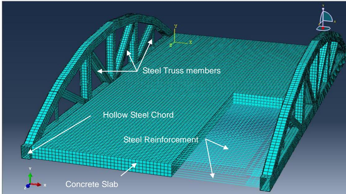
Fig. 6 Finite element mesh model
