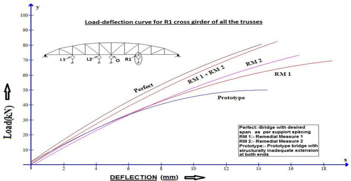
Fig. 9 Load deflection curve of 5 models at R1 Location
