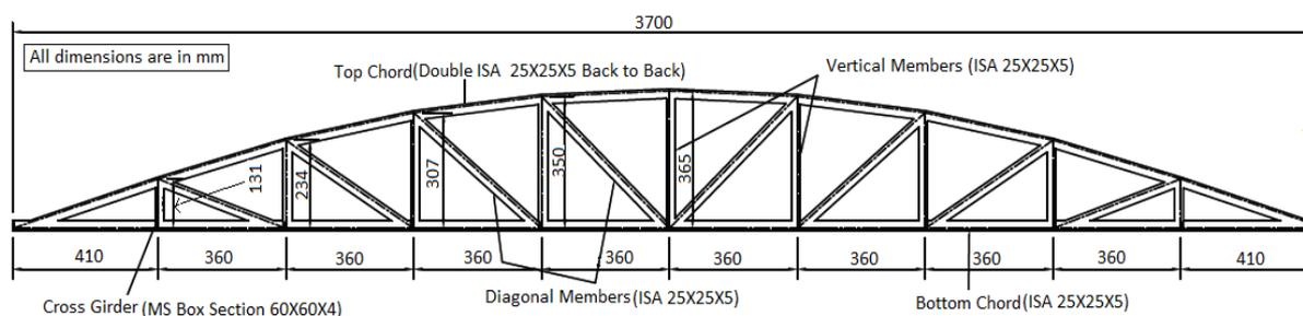
Fig. 4 Detailed figure of the bridge model
