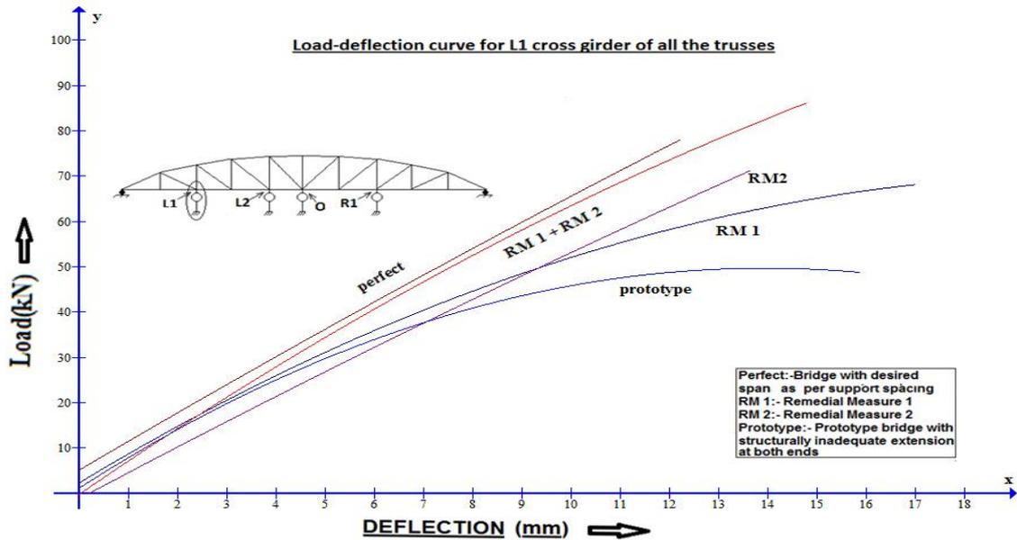
Fig. 10 Load deflection curve of 5 models at L1 location
