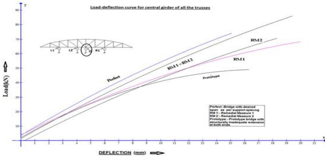
Fig. 7 Load deflection curve of 5 models at central location, O
