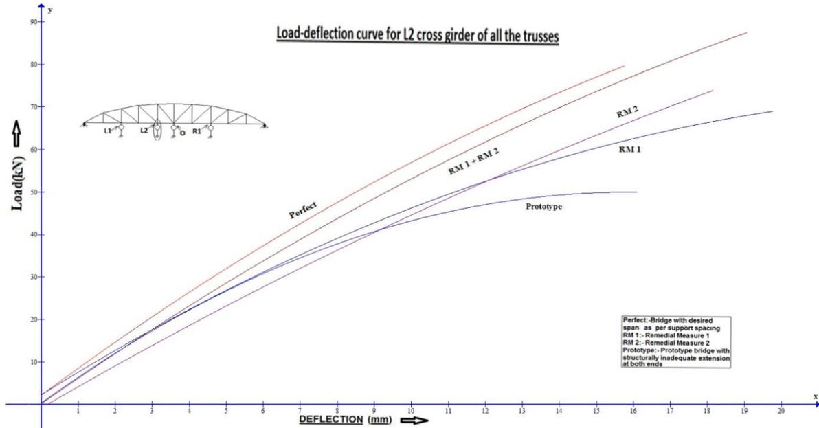
Fig. 8 Load deflection curve of 5 models at L2 location
