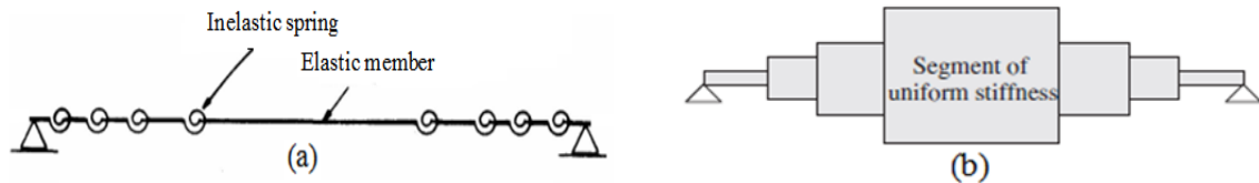
Fig. 2 Discrete element model (a) multi-spring model (Birely et al. 2012) (b) multi-section model (Wen and Janssen 1965)
