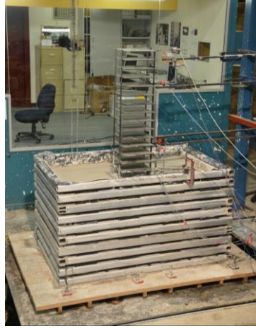
Fig. 7 Final setup of the measuring instruments of the soil-structure model
