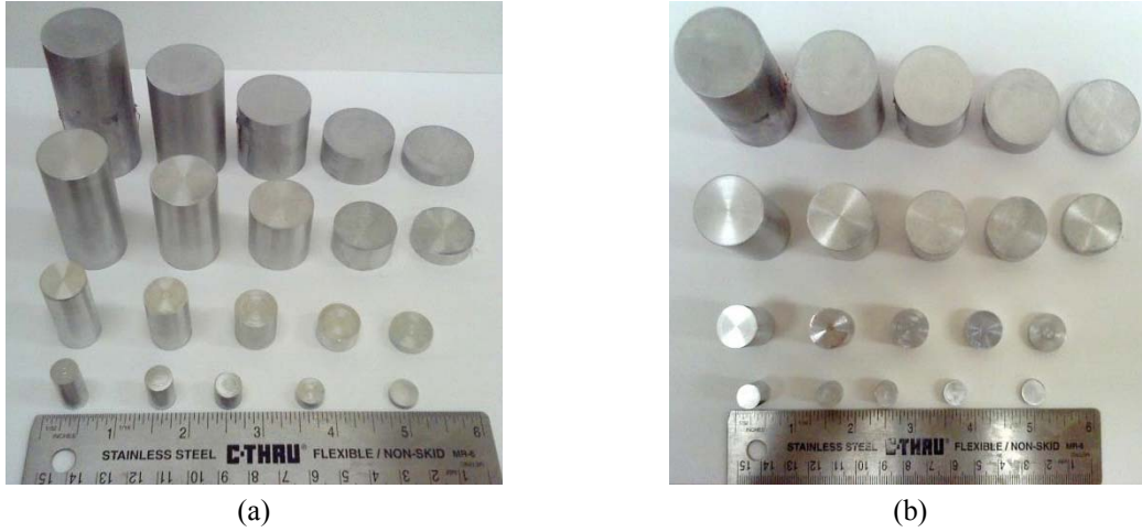
Fig. 2 Photo images of the aluminum 7075-T6 samples used for SHPB tests. (a) front view and (b) top view
