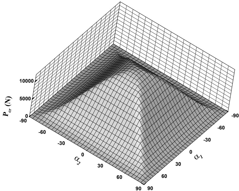
Fig. 4 Variation of axial buckling load of two joined conical shells versus semi-vertex cone angles  $\alpha_1$  and  $\alpha_2$
