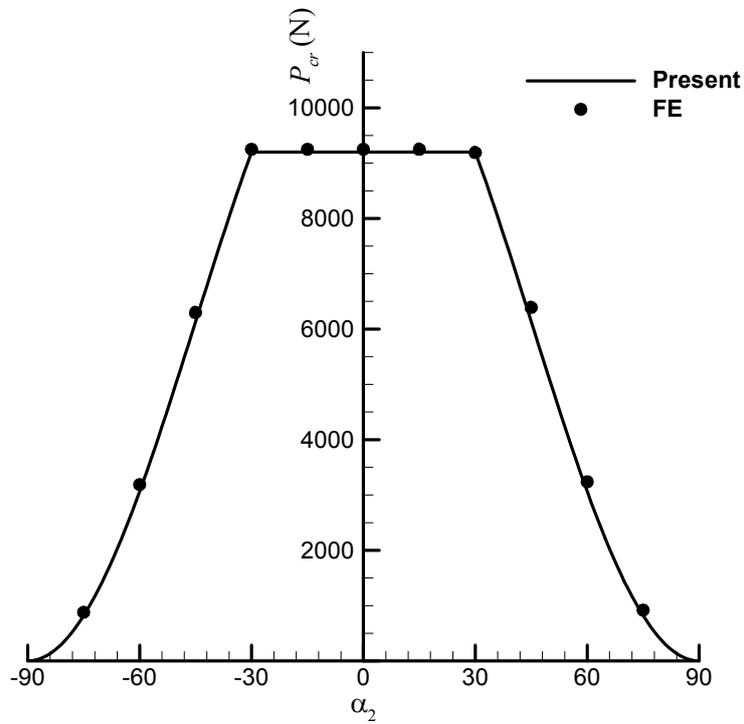
Fig. 2 Variation of axial buckling load of two joined conical shells versus  $\alpha_2$ : FE and present results ( $\alpha_1=30^\circ$ ,  $L/R=1$ )
