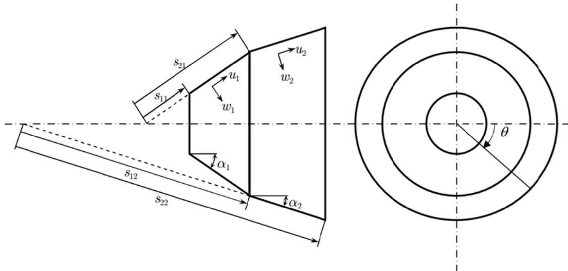
Fig. 1 Geometry of joined conical shells
