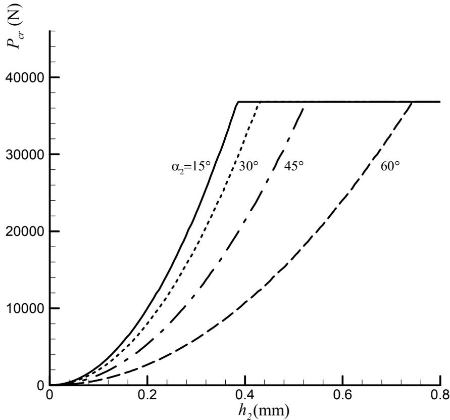
Fig. 5 Variation of axial buckling load of joined steel and aluminum conical shells versus aluminum cone thickness ( $\alpha_1=30^\circ$ ,  $L/R=1$  and  $h_1=0.254$  mm)
