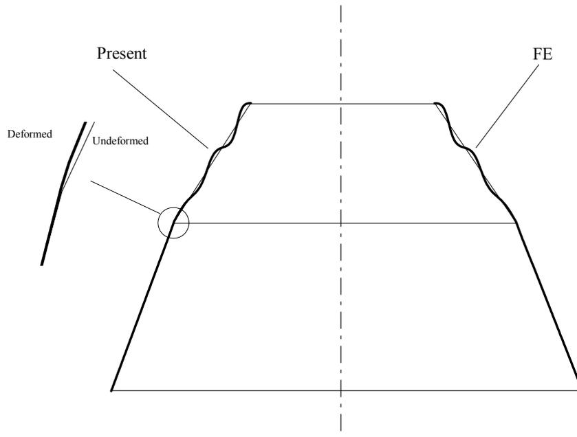
Fig. 3 Mode shape of two joined conical shells obtained from FE and present analysis ( $\alpha_1=45^\circ$ ,  $\alpha_2=30^\circ$ ,  $L/R=1$ )
