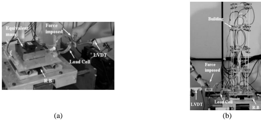
Fig. 7 Tests for the characterization of the restoring force of the RB
