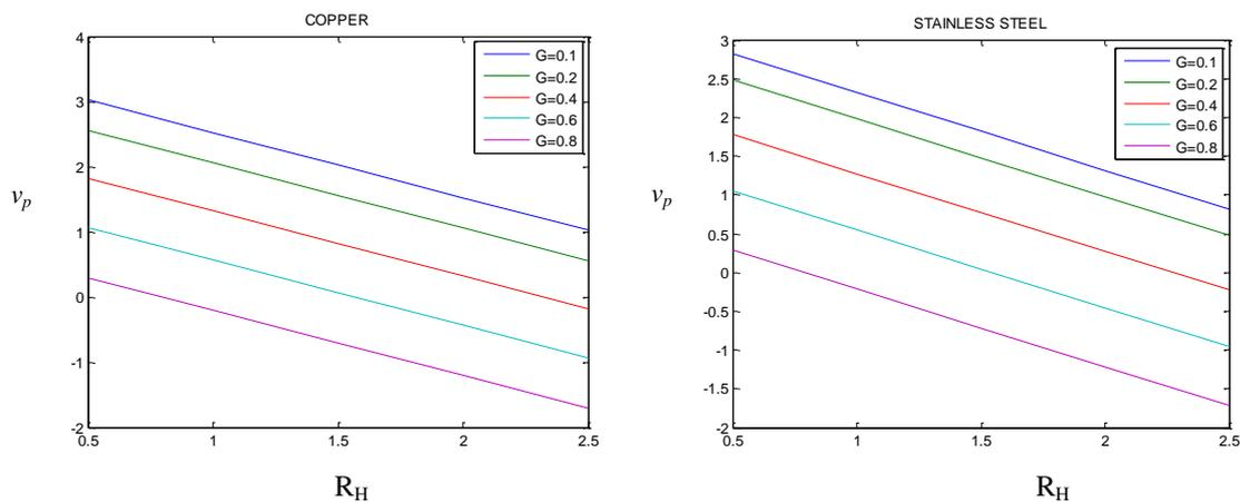
Fig. 3 Variation of  $v_p = \frac{c^2}{\beta_2^2}$  (phase velocity) of edge waves with  $R_H = \frac{c_a^2}{c_0^2}$  (electro-magneto pressure number) for different values of  $G = \zeta = \frac{P}{2\mu}$  (initial stress parameter) at constant  $\varepsilon$  (thermoelastic coupling parameter) for stainless steel and copper
