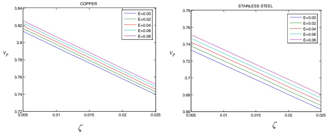
Fig. 5 Variation of  $v_p = \frac{c^2}{\beta_2^2}$  (phase velocity) of edge waves with  $\zeta = \frac{P}{2\mu}$  (initial stress parameter) for different values of  $\varepsilon$  (thermoelastic coupling parameter) keeping  $R_H = \frac{c_a^2}{c_0^2}$  (electro-magneto pressure number) constant for stainless steel and copper.
