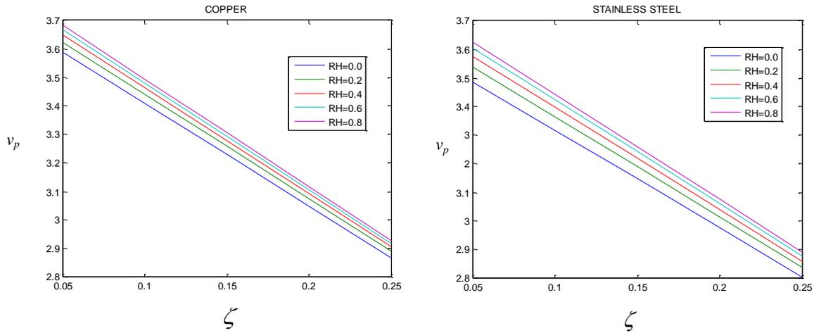
Fig. 2 Variation of  $v_p = \frac{c^2}{\beta_2^2}$  (phase velocity) of edge waves with  $\zeta = \frac{P}{2\mu}$  (initial stress parameter) for different values of  $R_H = \frac{c_a^2}{c_0^2}$  (electro-magneto pressure number) at constant  $\varepsilon$  (thermoelastic coupling parameter) for copper and stainless steel
