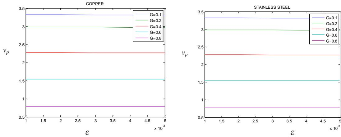
Fig. 4 Variation of  $v_p = \frac{c^2}{\beta_2^2}$  (phase velocity) of edge waves with  $\epsilon$  (thermoelastic coupling parameter) for different values of  $G = \zeta = \frac{P}{2\mu}$  (initial stress parameter) at constant  $R_H = \frac{c_a^2}{c_0^2} = 0.7$  (electro-magneto pressure number) for stainless steel and copper
