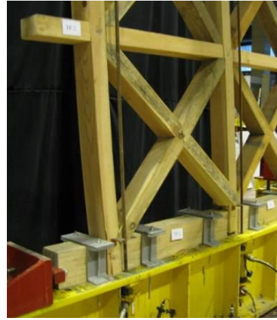
(b) Failure by compression and lateral instability of diagonal in TF2
