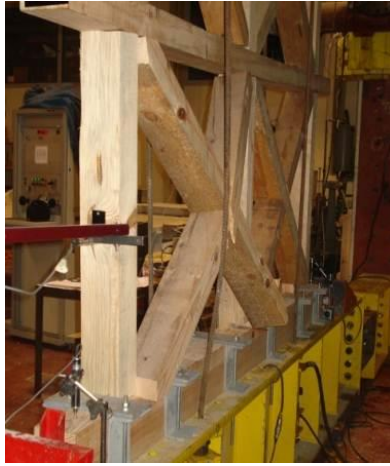
(a) Failure by compression and lateral instability of diagonal in TF1
