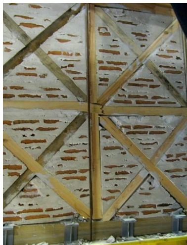
(a) Failure by shear of intermediate timber beam in MW1
