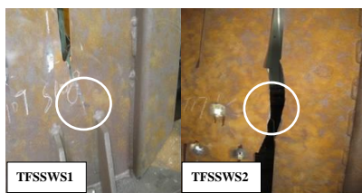
D: Extension of fracture at slits
