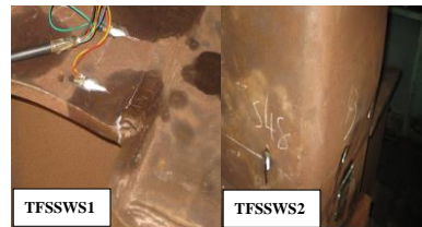
D: Fracture at beam flanges and inelastic deformation of column base
