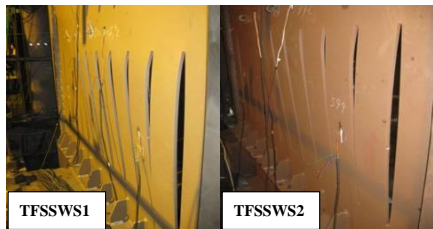
C: Development of out-plane deformation of flexural links in SSWs
