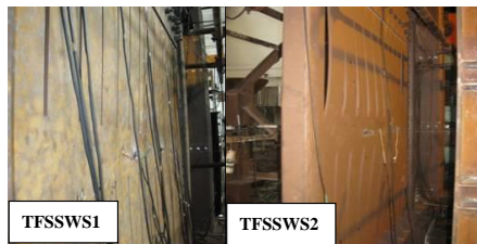
A: Initiation of out-plane deformation of flexural links in SSWs
