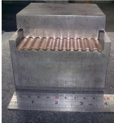
Fig. 2 Grooved die and copper sheet after the first groove pressing of CGP
