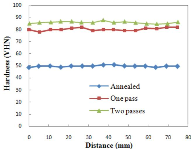
Fig. 7 The distribution of hardness measurements for specimens at each pass number
