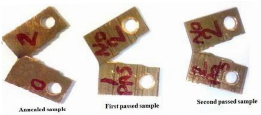
Fig. 9 CT specimens after fracture tests
