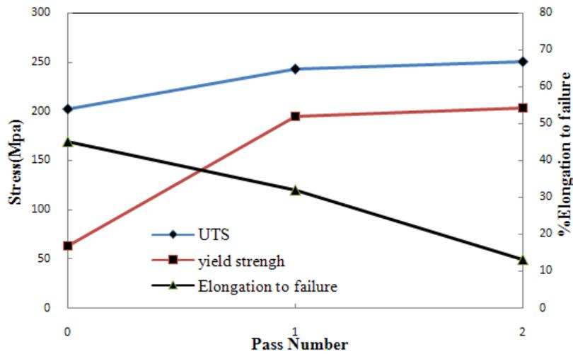
Fig. 6 Tensile properties of different CGPed pass of copper sheets
