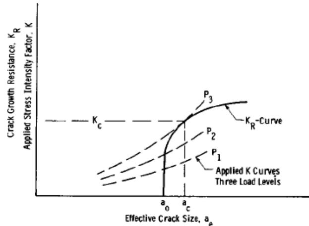
Fig. 5 Schematic  $R$ -curve;  $K_C$  occurs at the point of tangency between the applied  $K$ -curves at different load level and  $R$ -curve
