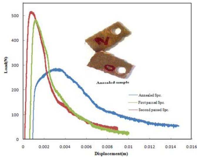
Fig. 10 Typical load-displacement curves in the CT tests of the annealed, first and second passed Cu specimens
