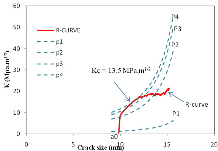
Fig. 11 *R* curve for annealed specimen
