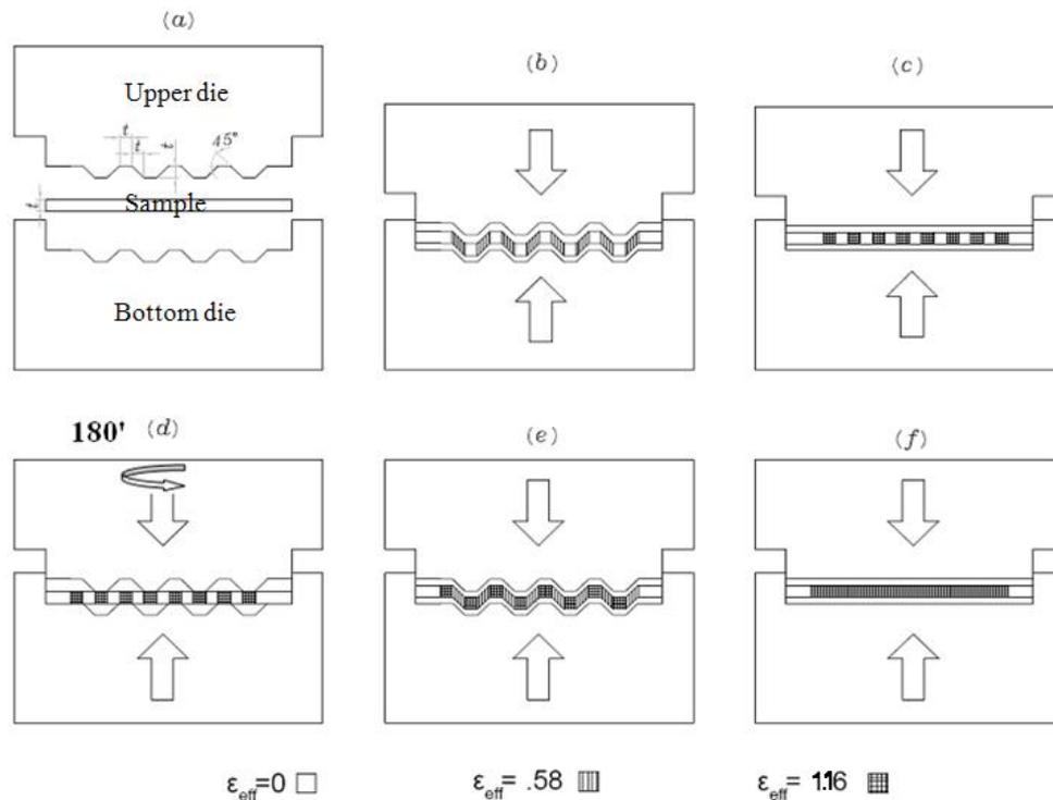
Fig. 1 A schematic illustration of the sequences of the constrained groove pressing (CGP)
