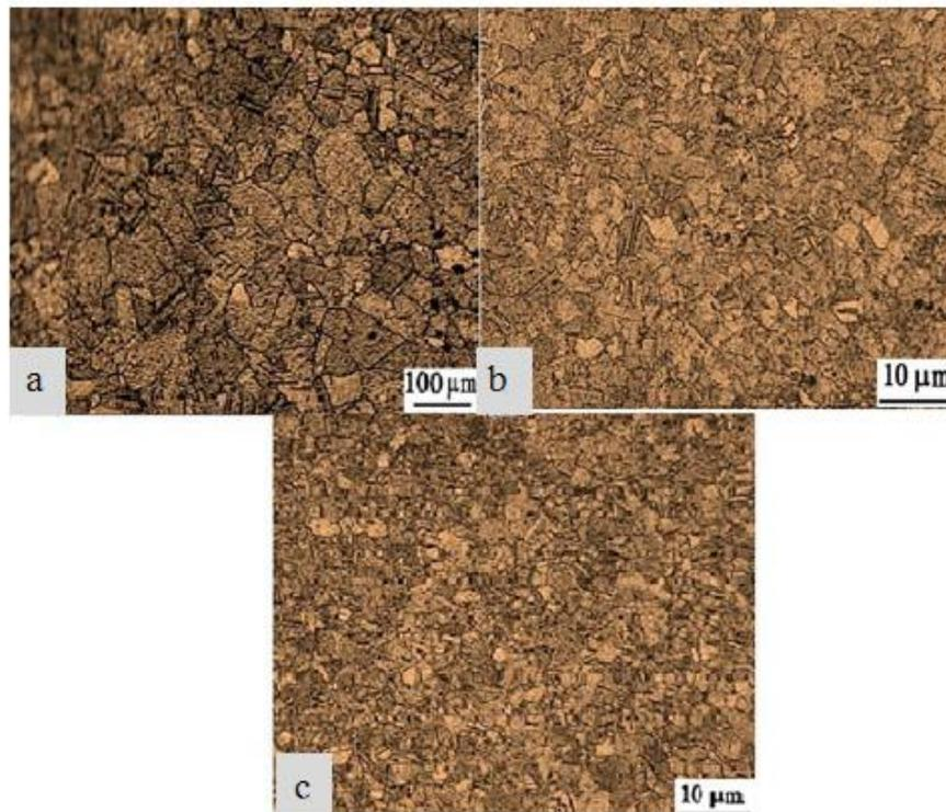
Fig. 8 Optical microscope (OM) microstructure of the commercially pure copper subjected to groove pressing specimens (a) as-received Cu specimen (b) OM micrograph after one pass (c) OM micrograph after three passes
