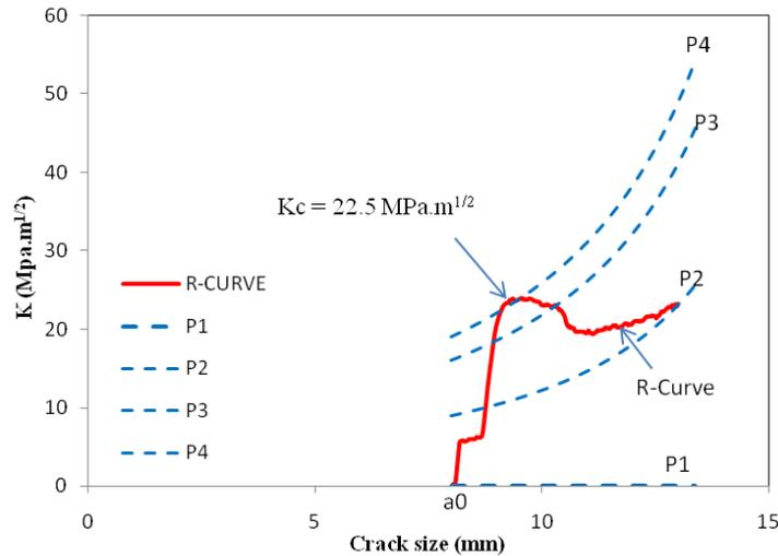
Fig. 13 R curve for second passed specimen
