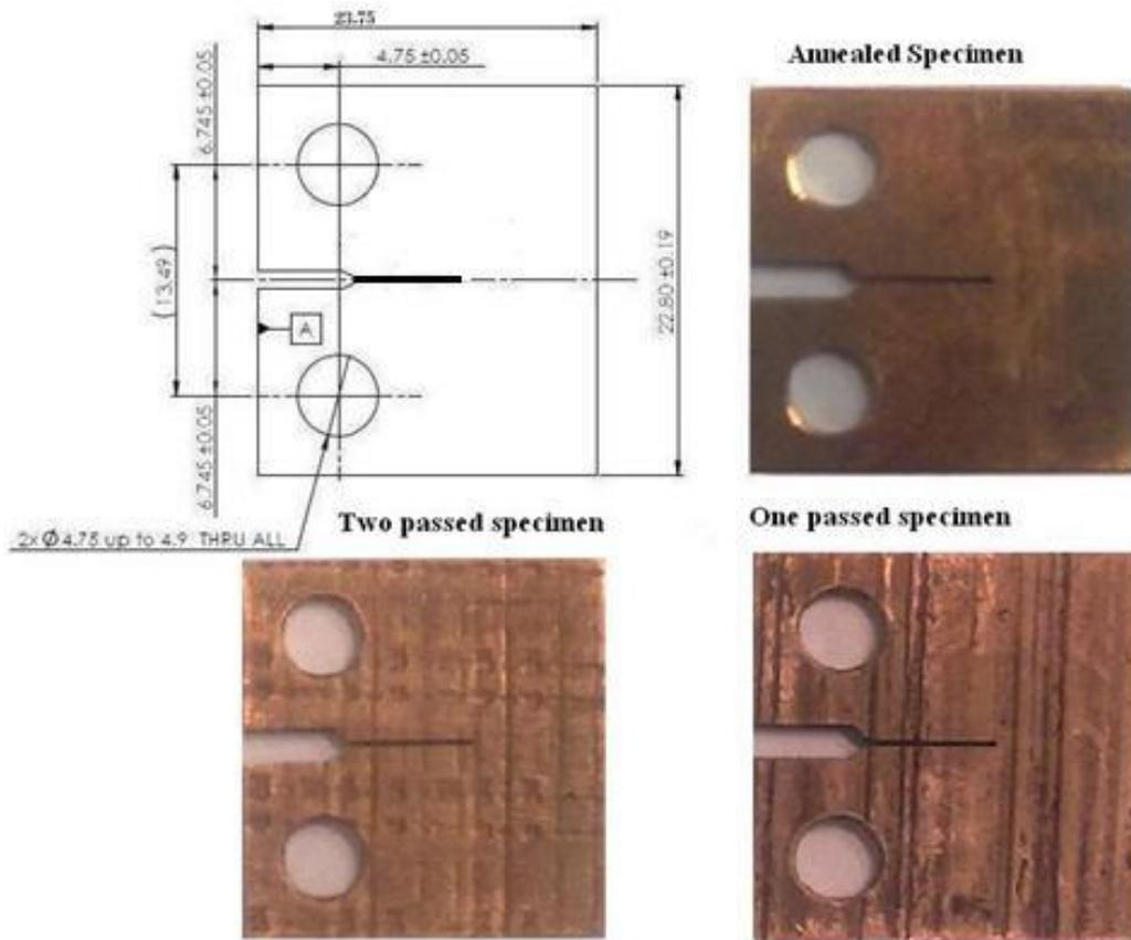
Fig. 3 Annealed, one, and two passed CT specimens of CGPed copper
