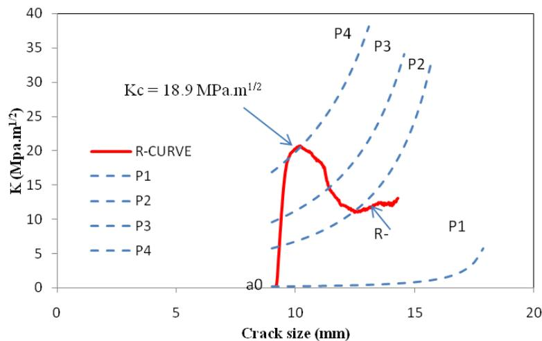
Fig. 12 *R* curve for first passed specimen
