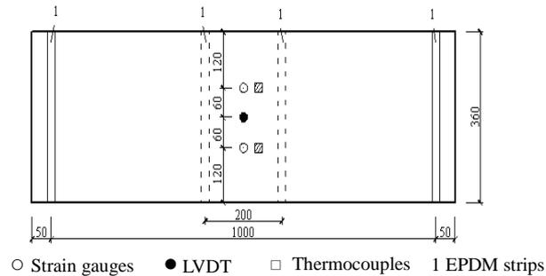
Fig. 2 Layout of measuring instruments
