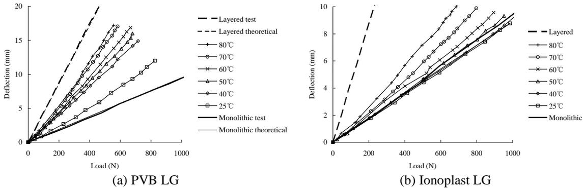
Fig. 4 Load-deflection curves of the specimens
