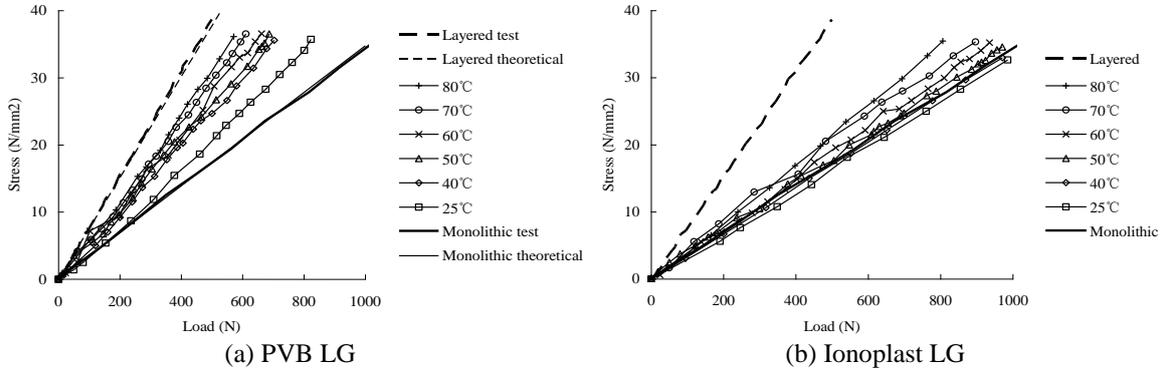
Fig. 3 Load-stress curves of the specimens
