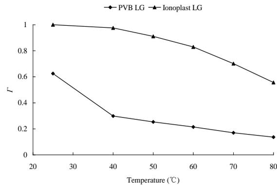
Fig. 6 Shear transfer coefficients of PVB and Ionoplast LG
