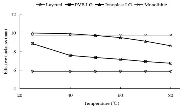
Fig. 5 Effective thicknesses for the PVB and Ionoplast LG in different ambient temperatures
