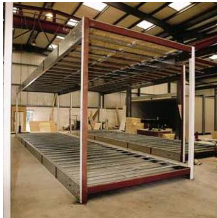
(a) A typical primary steel frame
