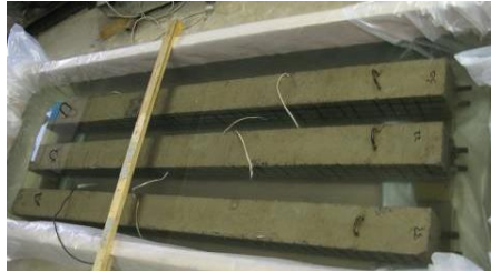
Fig. 4 Specimens immersing in the acid solution
