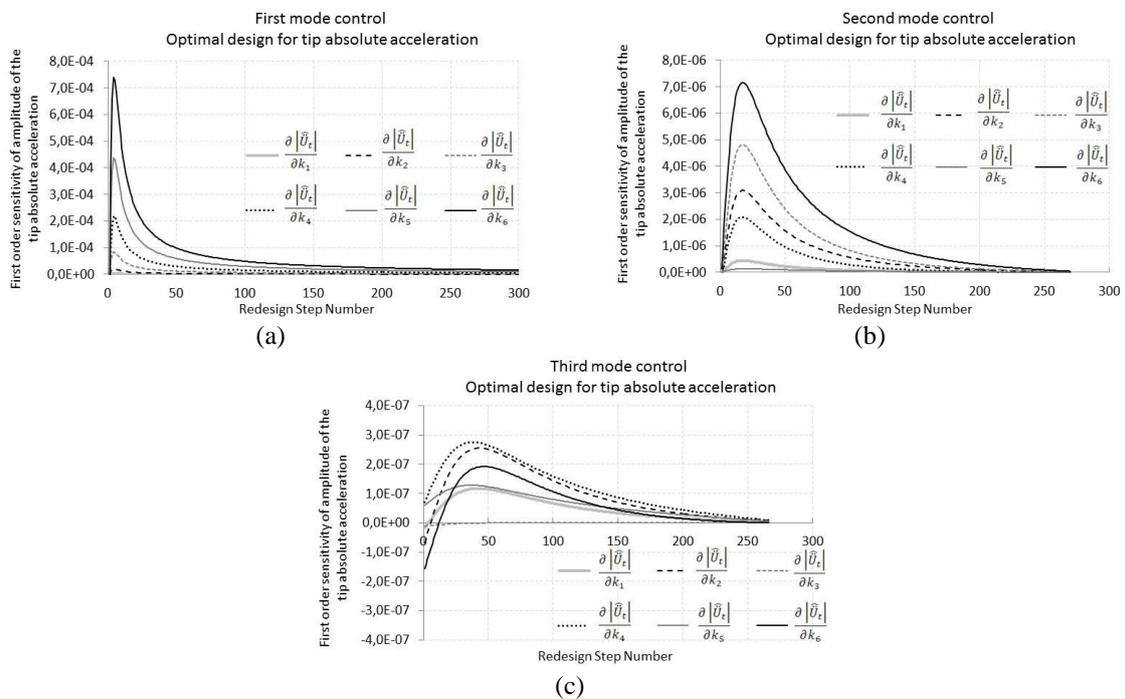
Fig. 7 Variation of the first order sensitivity of the amplitude of tip absolute acceleration with respect to redesign step number in the first-three modes
