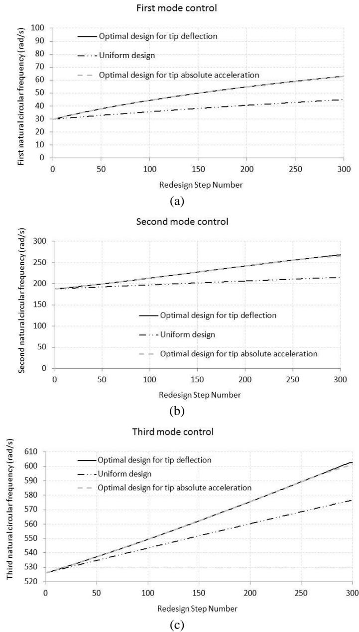
Fig. 5 Variation of natural circular frequency with respect to redesign step number in the first-three modes
