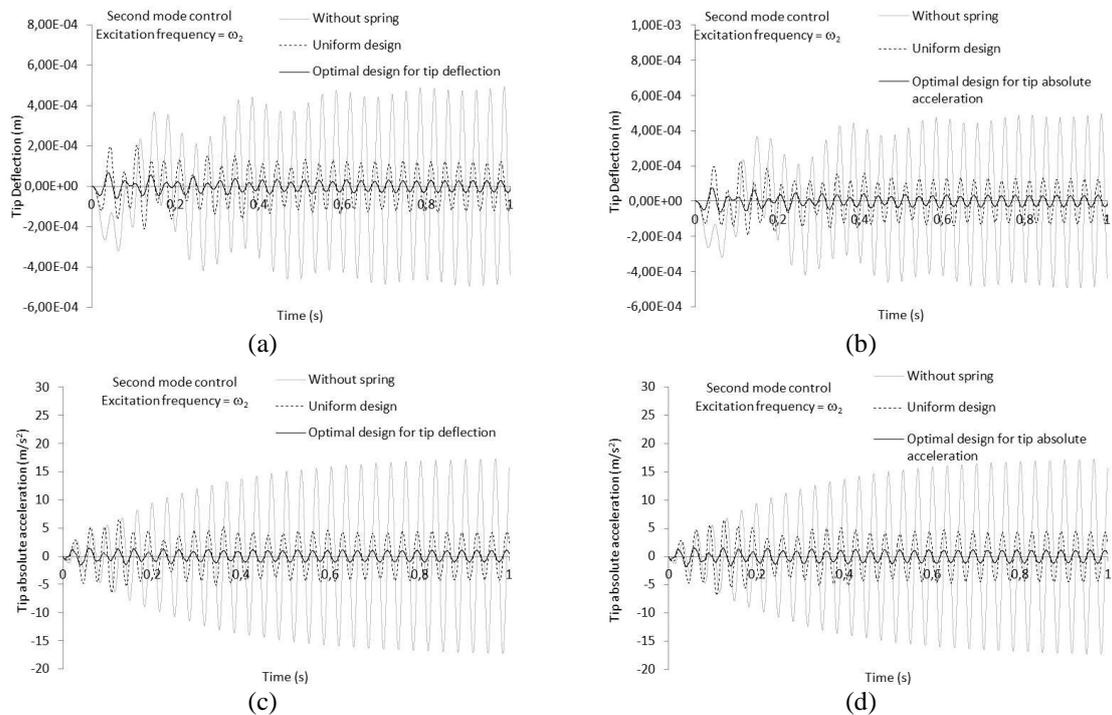
Fig. 11 Time history of the tip deflection of the beam under the sinusoidal base excitation for the second mode control
