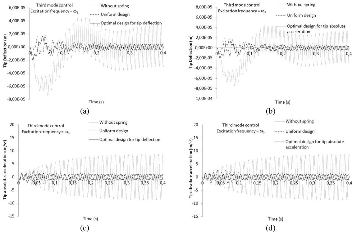
Fig. 12 Time history of the tip deflection of the beam under the sinusoidal base excitation for the third mode control
