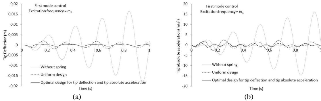
Fig. 10 Time history of the tip deflection of the beam under the sinusoidal base excitation for the first mode control
