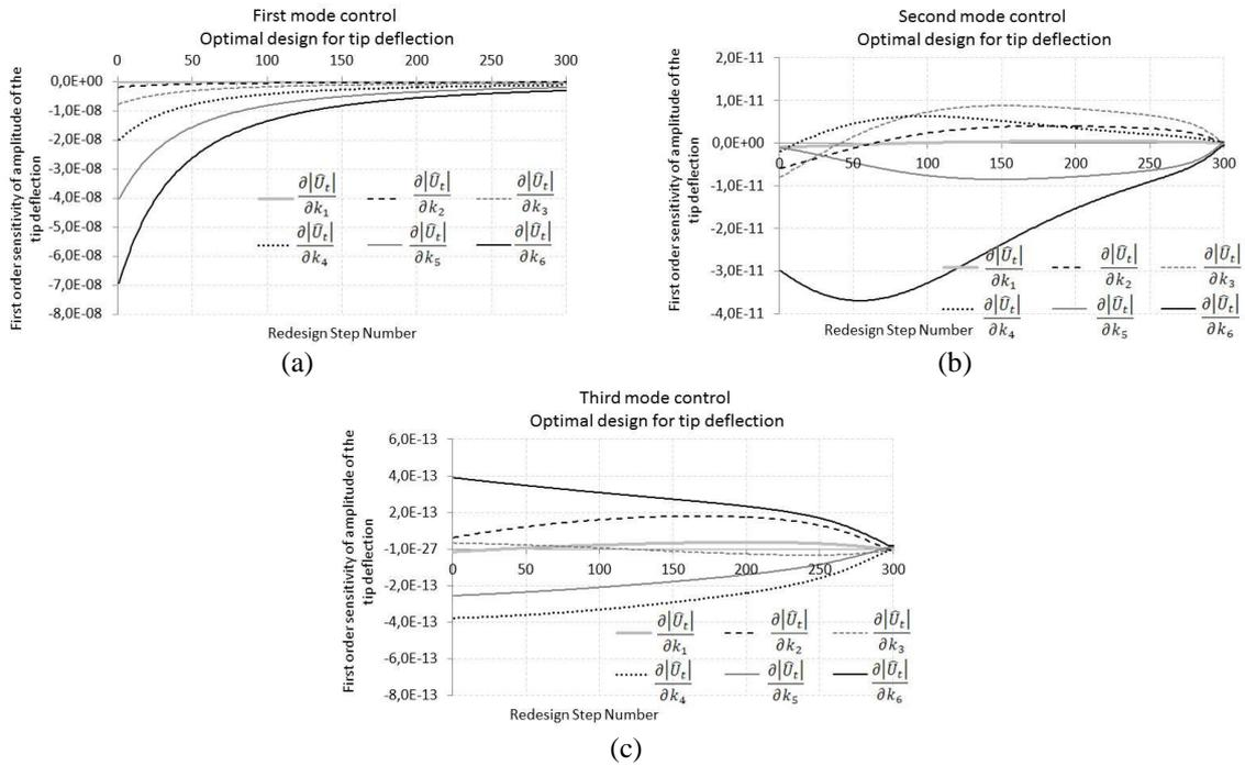
Fig. 6 Variation of the first order sensitivity of the amplitude of tip deflection with respect to redesign step number in the first-three modes
