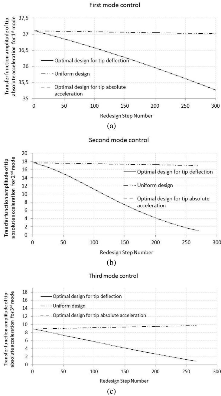
Fig. 4 Variation of objective function for tip absolute acceleration with respect to redesign step number in the first-three modes
