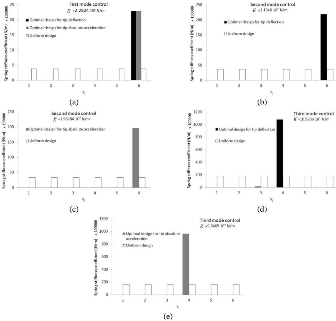
Fig. 2 Optimal spring designs for first-three modes
