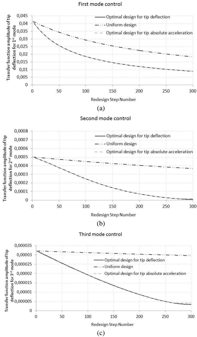
Fig. 3 Variation of objective function for tip deflection with respect to redesign step number in the first-three modes
