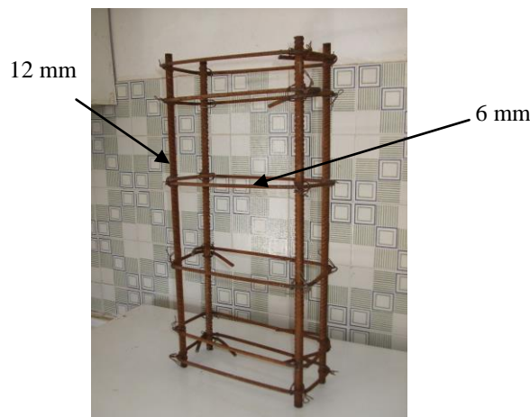
Fig. 2 Geometry of specimens and reinforcement cage (unit: mm; 1 mm = 0.039 in)
