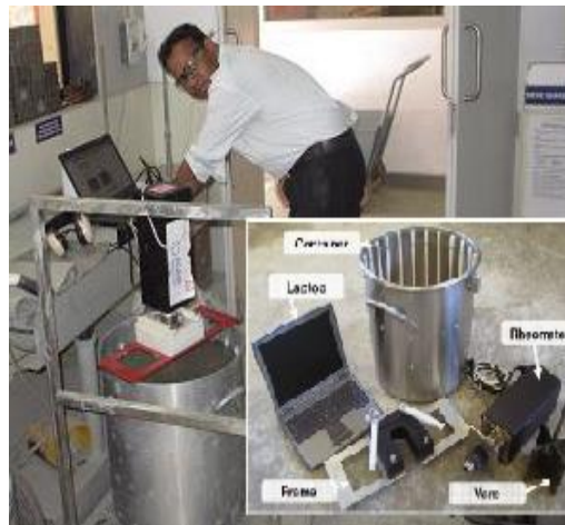
Fig. 1 ICAR Rheometer testing and set-up
