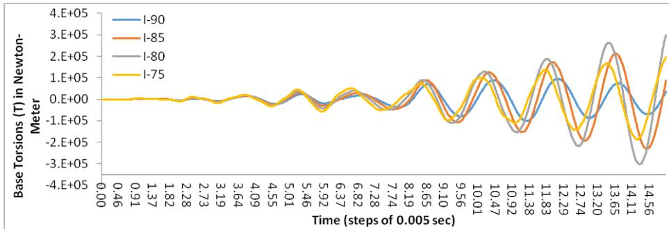
Fig. 22 Base torsions (T) for earthquake excitation, I-type column supports
