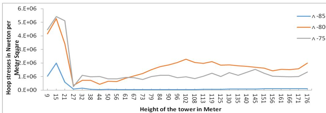
Fig. 13 Hoop stresses along the height of the tower at  $\theta=0^\circ$  for  $\Lambda$ -type column supports
