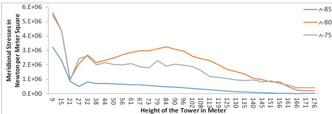
Fig. 11 Meridian stresses along the height of the tower at  $\theta=0^\circ$  for  $\Lambda$ -type column supports
