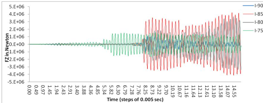
Fig. 16 Base reactions (FZ) for earthquake excitation, I-type column supports
