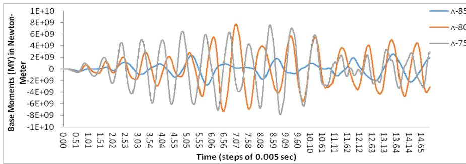
Fig. 21 Base reactions (MY) for earthquake excitation, Λ-type column supports
