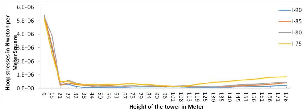
Fig. 12 Hoop stresses along the height of the tower at  $\theta=0^\circ$  for I-type column supports
