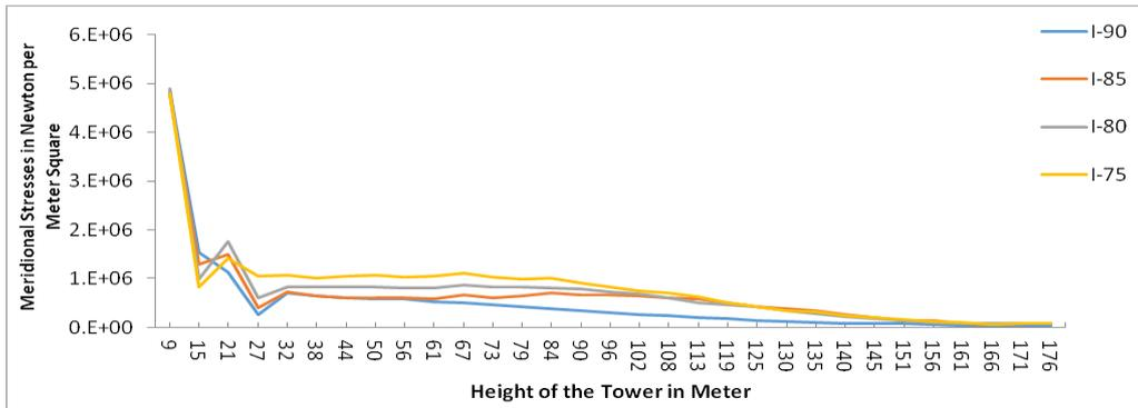
Fig. 10 Meridian stresses along the height of the tower at  $\theta=0^\circ$  for I-type column supports
