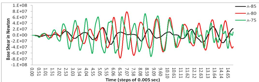
Fig. 15 Base shear force under earthquake excitation for  $\Lambda$ -type column supports
