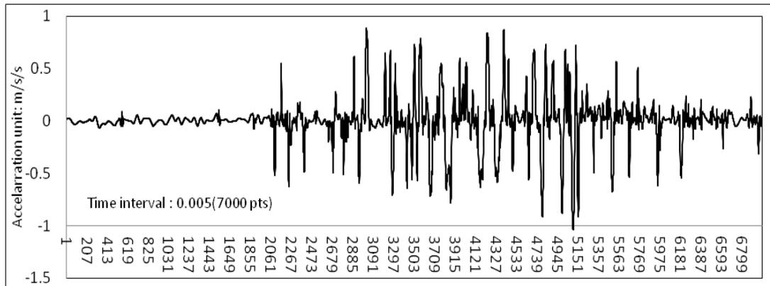
Fig. 3 Earthquake records (accelerations in  $\text{m/sec}^2$ ) of Bhuj city
