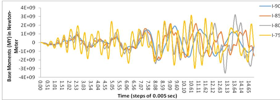
Fig. 20 Base reactions (MY) for earthquake excitation, I-type column supports
