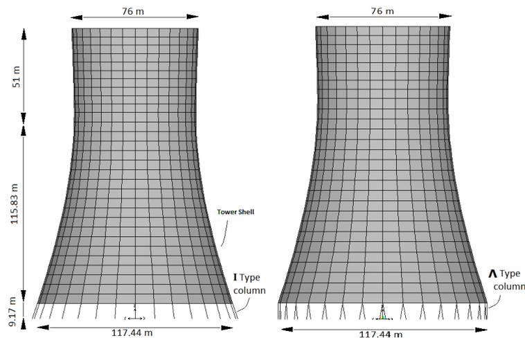
Fig. 1 Geometrical representation and analytical model of tower
