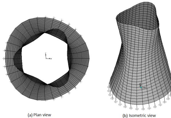
Fig. 4 Circumferential mode having three waves in the highest period of vibration
