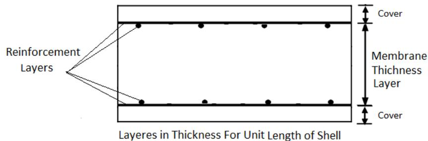
Fig. 2 Layered shell element to model the different layers of concrete and reinforcement
