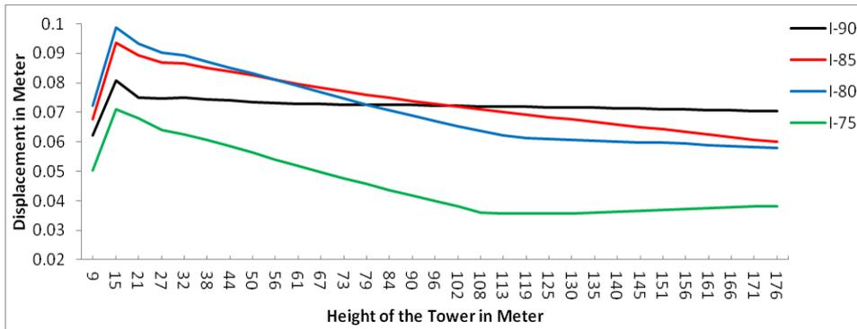
Fig. 8 Maximum radial displacements along the tower height at  $\theta=0^\circ$  at m1 for I-type column supports
