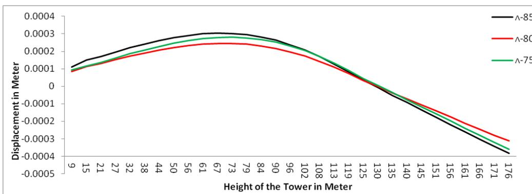
Fig. 7 Vibration modes for the highest period of the  $\Lambda$ -type column supports at m1
