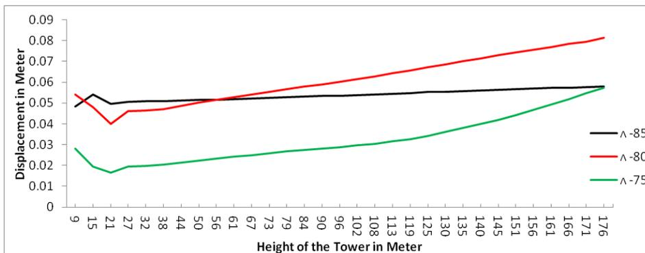
Fig. 9 Maximum radial displacements along the tower height at  $\theta=0^\circ$  at m1 for  $\Lambda$ -type column supports
