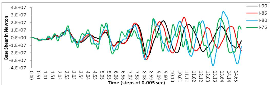
Fig. 14 Base shear force under earthquake excitation for I-type column supports
