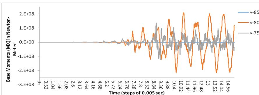
Fig. 19 Base reactions (MY) for earthquake excitation, Lambda-type column supports
