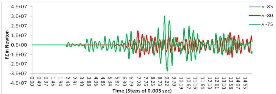
Fig. 17 Base reactions (FZ) for earthquake excitation, Lambda-type column supports
