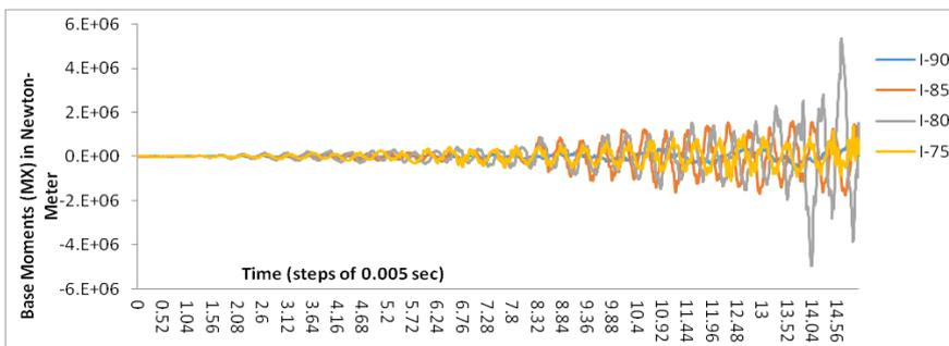
Fig. 18 Base reactions (MX) for earthquake excitation, I-type column supports
