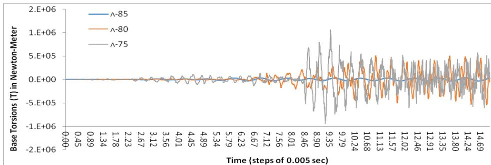
Fig. 23 Base torsions (T) for earthquake excitation, Λ-type column supports
