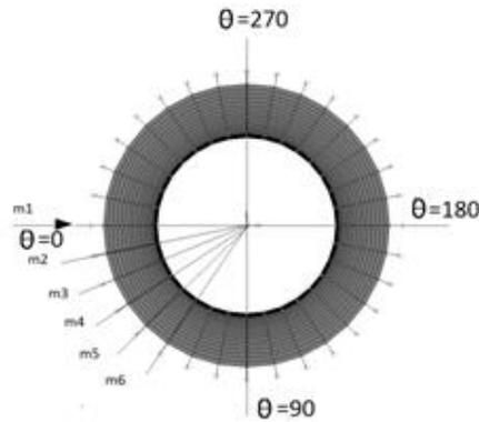
Fig. 5 Key diagrams to plot the axial modes varying by  $11.25^\circ$  from m1 to m2
