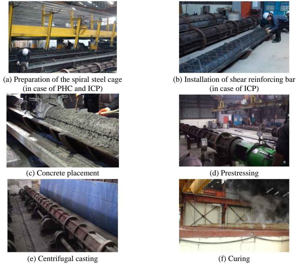
Fig. 1 Manufacturing procedures of PHC and ICP pile
