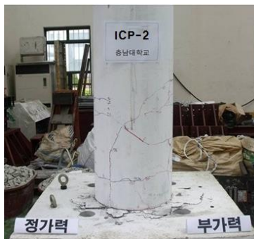
Fig. 7 Crack and failure patterns of the each specimen
