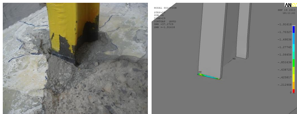
Fig. 9 Debonding, took place at the interface of steel column-RC base
