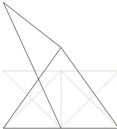
Fig. 7 Optimum topology and geometry of a ten bar planar truss
