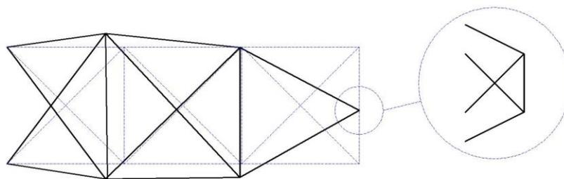
Fig. 2 Optimum geometry of fifteen-bar truss
