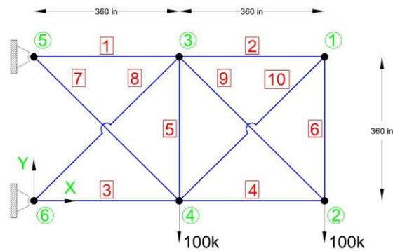
Fig. 6 The primary geometry and topology of a ten-bar truss
