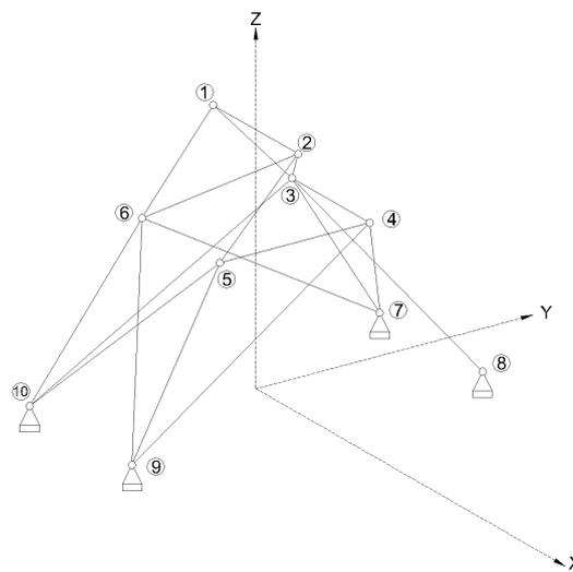
Fig. 9 Optimum topology and geometry of the twenty five-bar space truss
