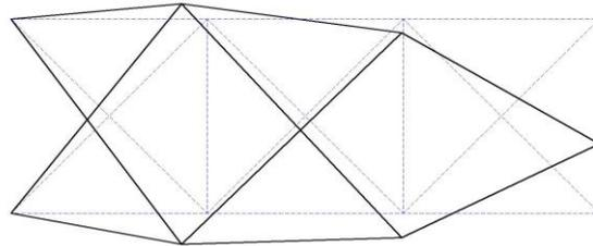
Fig. 8 Optimum topology and geometry of the fifteen-bar truss
