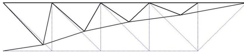
Fig. 4 The optimum geometry of eighteen-bar planar truss
