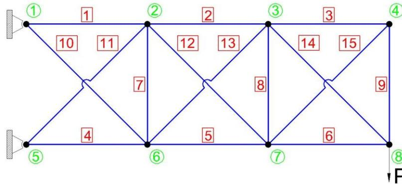
Fig. 1 The topology of a fifteen-bar truss
