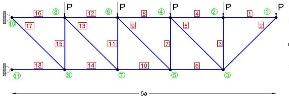
Fig. 3 The topology of an eighteen-bar planar truss ( $a=250$  in)
