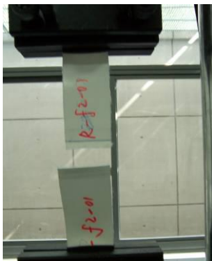
Welded layer slippage
