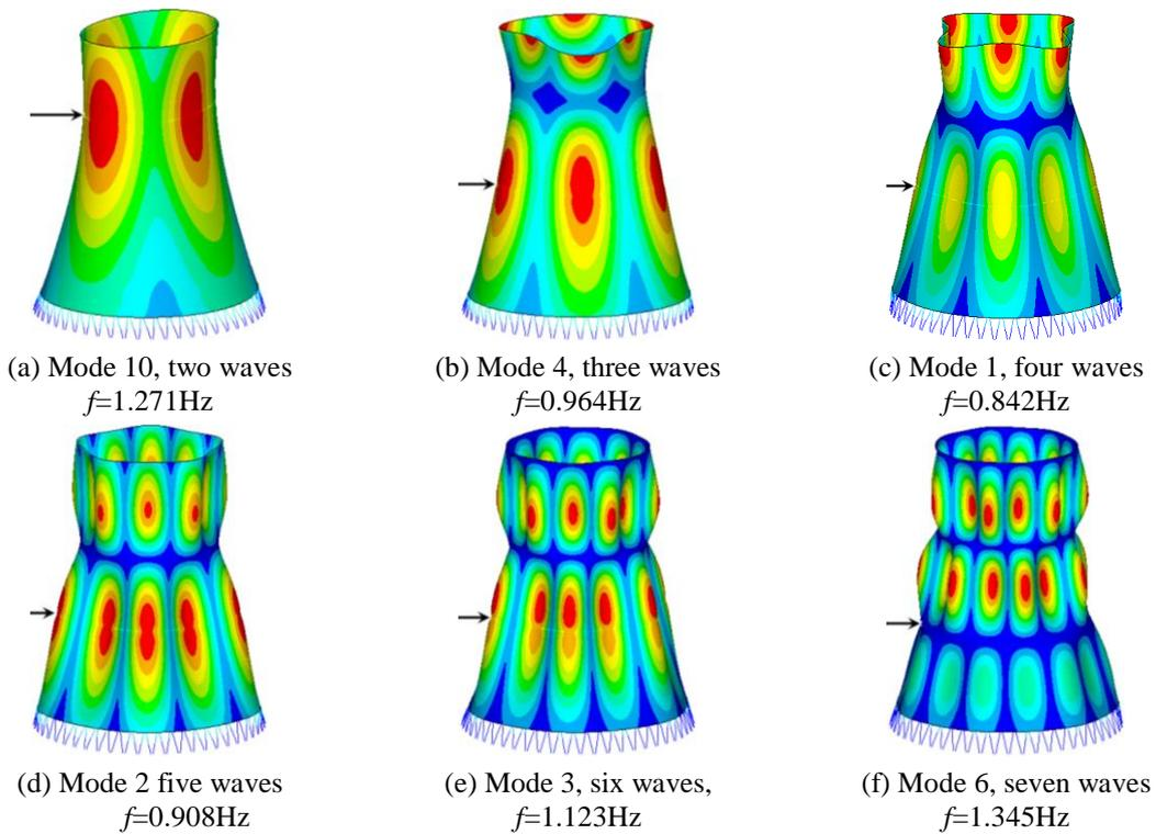
Fig. 8 Mode shapes of the stiffened cooling tower
