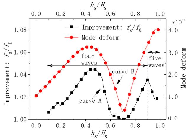
Fig. 5 Improvement of the fundamental eigenfrequency by one stiffening ring
