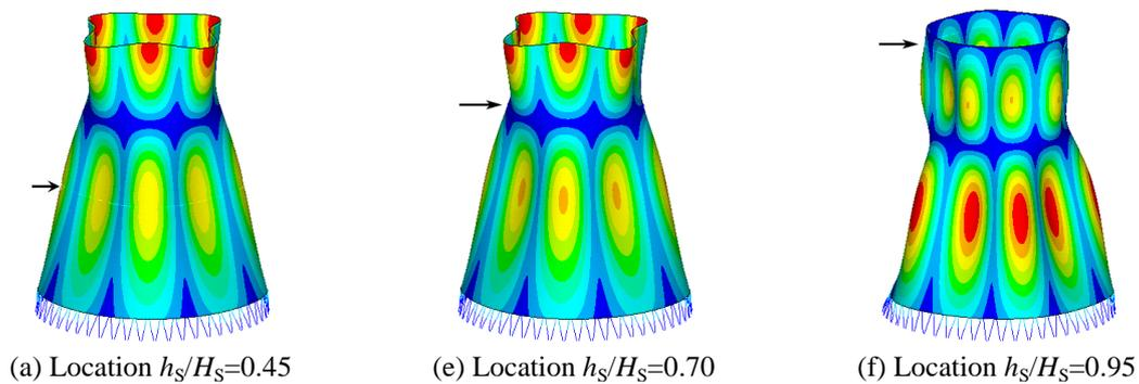
Fig. 6 Representative mode shapes for different locations of the stiffening ring
