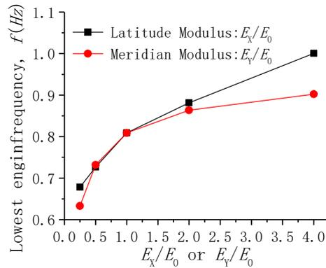
Fig. 4 Effects of stiffness in the two directions on the fundamental eigenfrequency
