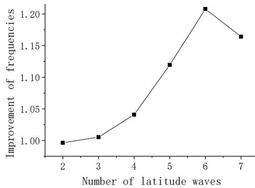
Fig. 7 Improvement of different mode eigenfrequencies by one stiffening ring
