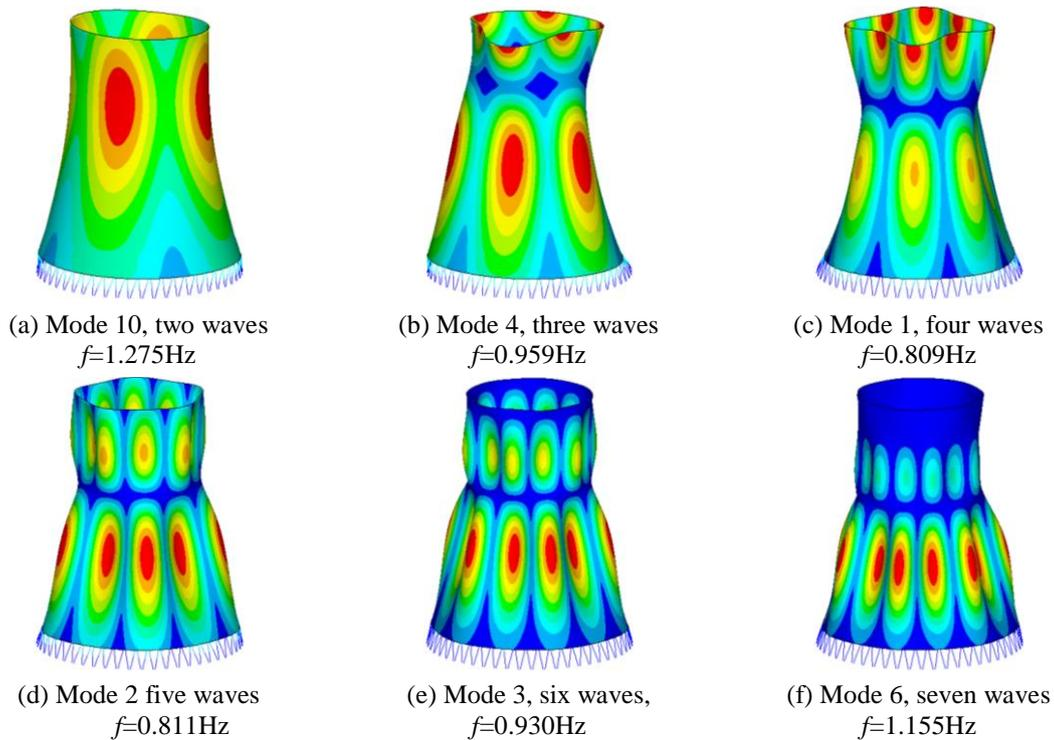
Fig. 2 Mode shapes of the unstiffened cooling tower
