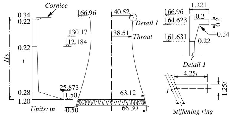
Fig. 1 Dimensions of the representative cooling tower
