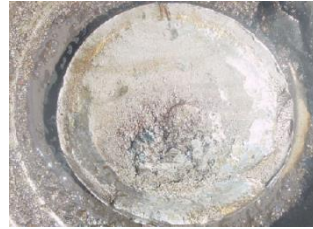
Fig. 1 Fracture at axle mounting point in a tank car caused by the fatigue and derailment (Locovei 2010)
