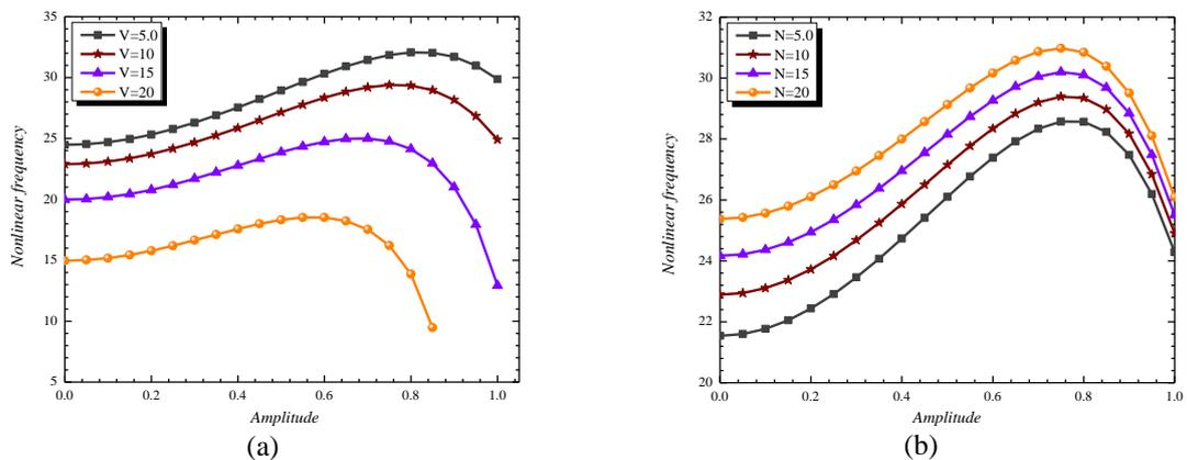
Fig. 4 Effect of (a)  $V$  parameter and (b)  $N$  parameter on nonlinear frequency of electrostatically microbeam base on amplitude
