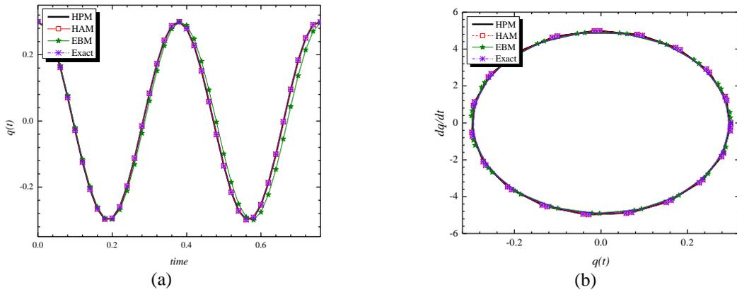
Fig. 2 Comparison of homotopy perturbation method (HPM), homotopy analysis method (HAM), energy balance method (EBM) and exact solution. (a) time history response, (b) phase plane for  $N=10$ ,  $\lambda=24$ ,  $V=20$ ,  $A=0.3$
