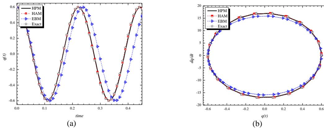
Fig. 3 Comparison of homotopy perturbation method (HPM), homotopy analysis method (HAM), energy balance method (EBM) and exact solution. (a) time history response, (b) phase plane for  $N=10$ ,  $\lambda=24$ ,  $V=10$ ,  $A=0.6$
