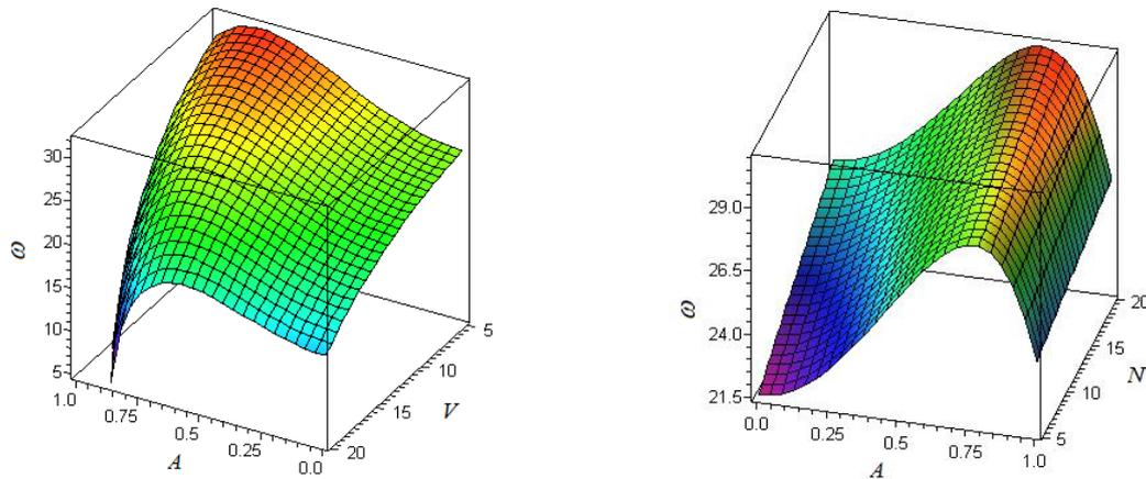
Fig. 5 Sensitivity analysis of nonlinear frequency for (a)  $N=10$ ,  $\lambda=24$ ,  $5 < V < 20$ ,  $0 < A < 1$  (b)  $5 < N < 20$ ,  $\lambda=24$ ,  $V=10$ ,  $0 < A < 1$
