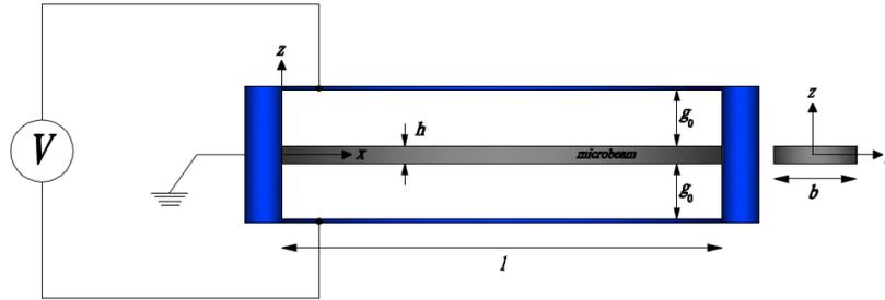
Fig. 1 Schematics of a double-sided driven clamped-clamped microbeam-based electromechanical resonator
