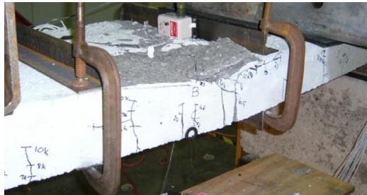
(a) Ductile failure for flexural specimen
