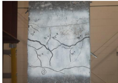
(c) Tension specimen failure mode
