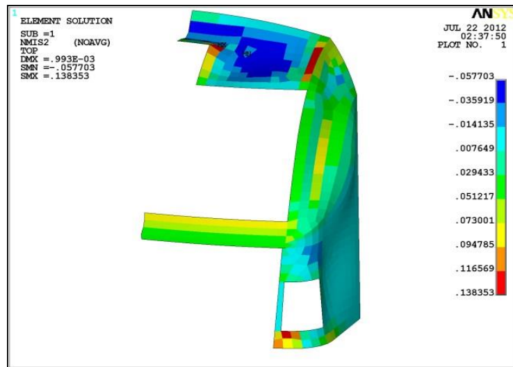
Fig. 12 Tsai-Wu criteria for the optimized composite frontend structure
