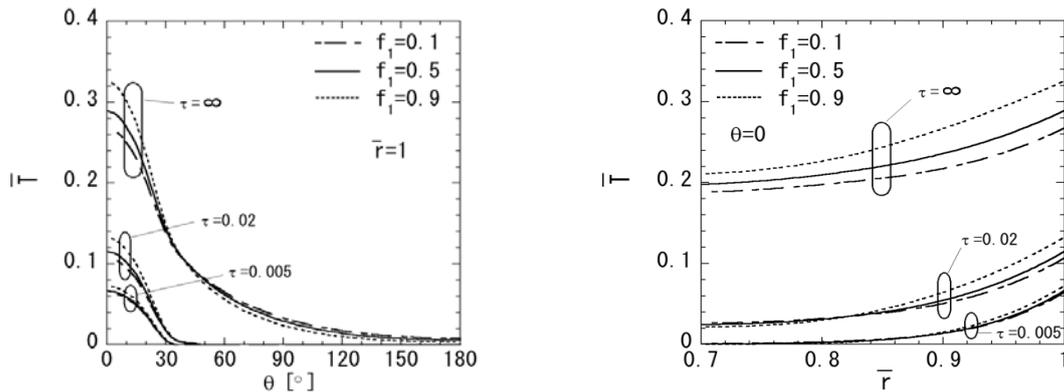
Fig. 1 Temperature change (Material 1,  $N = 2$ ,  $\bar{r}_1 = 0.85$ ): (a) variation in the heated surface ( $\bar{r} = 1.0$ ) and (b) variation in the radial direction ( $\theta = 0$ )
