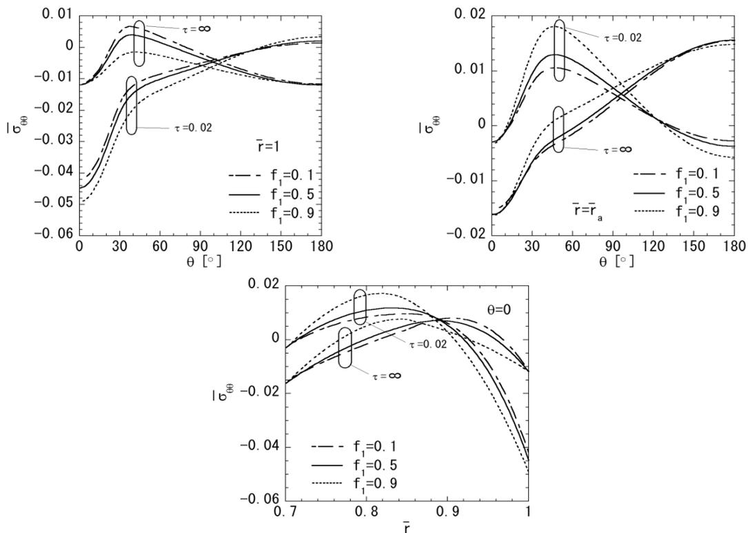
Fig. 2 Variation of thermal stress  $\bar{\sigma}_{\theta\theta}$  (Material 1,  $N = 2$ ,  $\bar{r}_1 = 0.85$ ): (a) variation in the heated surface ( $\bar{r} = 1.0$ ), (b) variation in the inner surface ( $\bar{r} = 0.7$ ) and (c) variation in the radial direction ( $\theta = 0$ )
