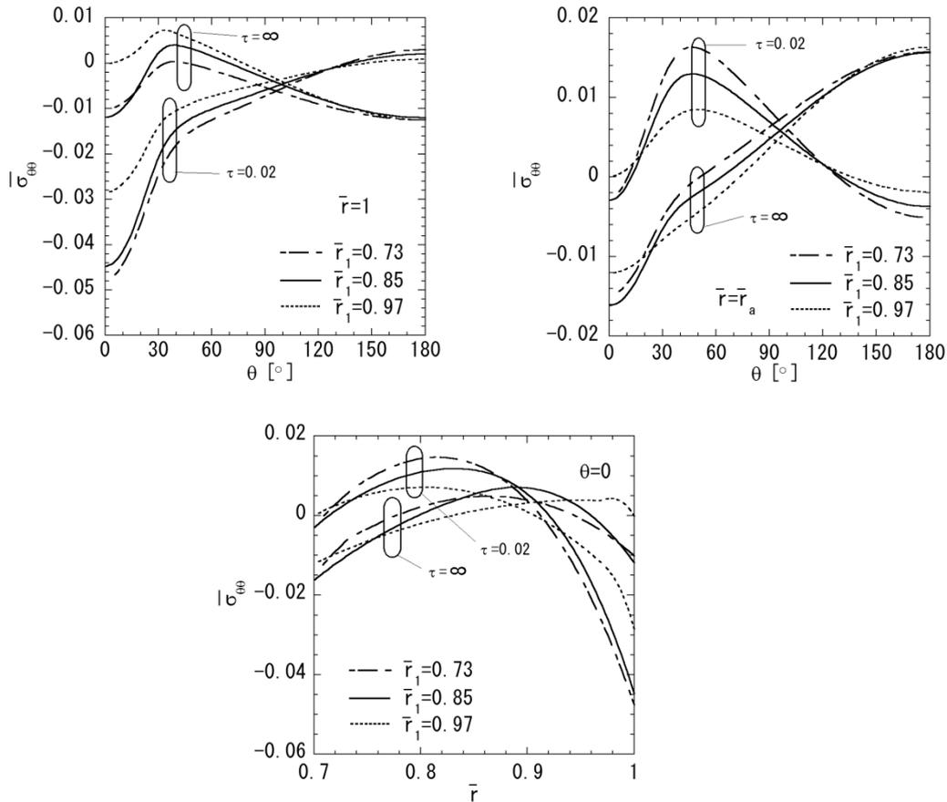
Fig. 5 Variation of thermal stress  $\bar{\sigma}_{\theta\theta}$  (Material 2,  $N = 2, f_1 = 0.5$ ): (a) variation in the heated surface ( $\bar{r}_1 = 1.0$ ), (b) variation in the inner surface ( $\bar{r} = 0.7$ ) and (c) variation in the radial direction ( $\theta = 0$ )
