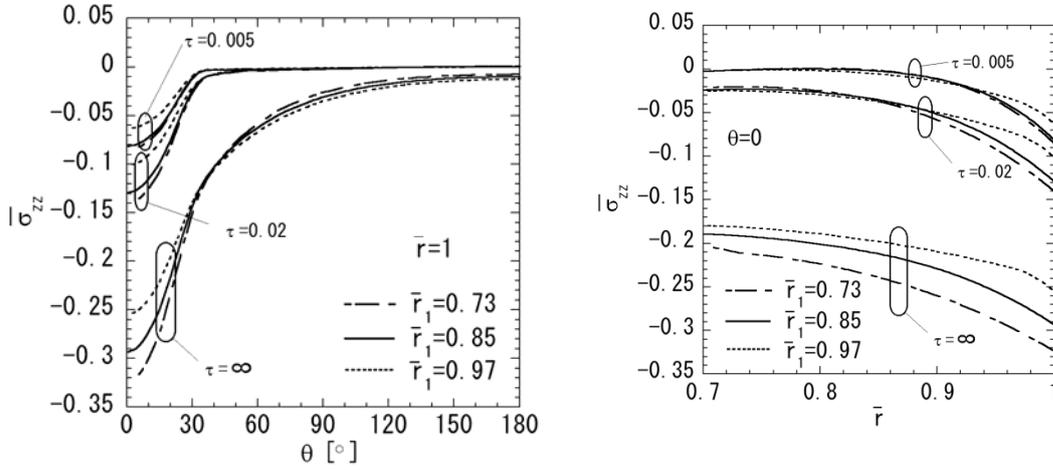
Fig. 6 Variation of thermal stress  $\bar{\sigma}_{zz}$  (Material 2,  $N = 2, f_1 = 0.5$ ): (a) variation in the heated surface ( $\bar{r} = 1.0$ ) and (b) variation in the radial direction ( $\theta = 0$ )
