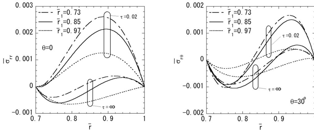
Fig. 7 Variation of thermal stresses in the radial direction (Material 2,  $N = 2, f_1 = 0.5$ ): (a) normal stress  $\bar{\sigma}_{rr}$  ( $\theta = 0$ ) and (b) shearing stress  $\bar{\sigma}_{r\theta}$  ( $\theta = 30^\circ$ )
