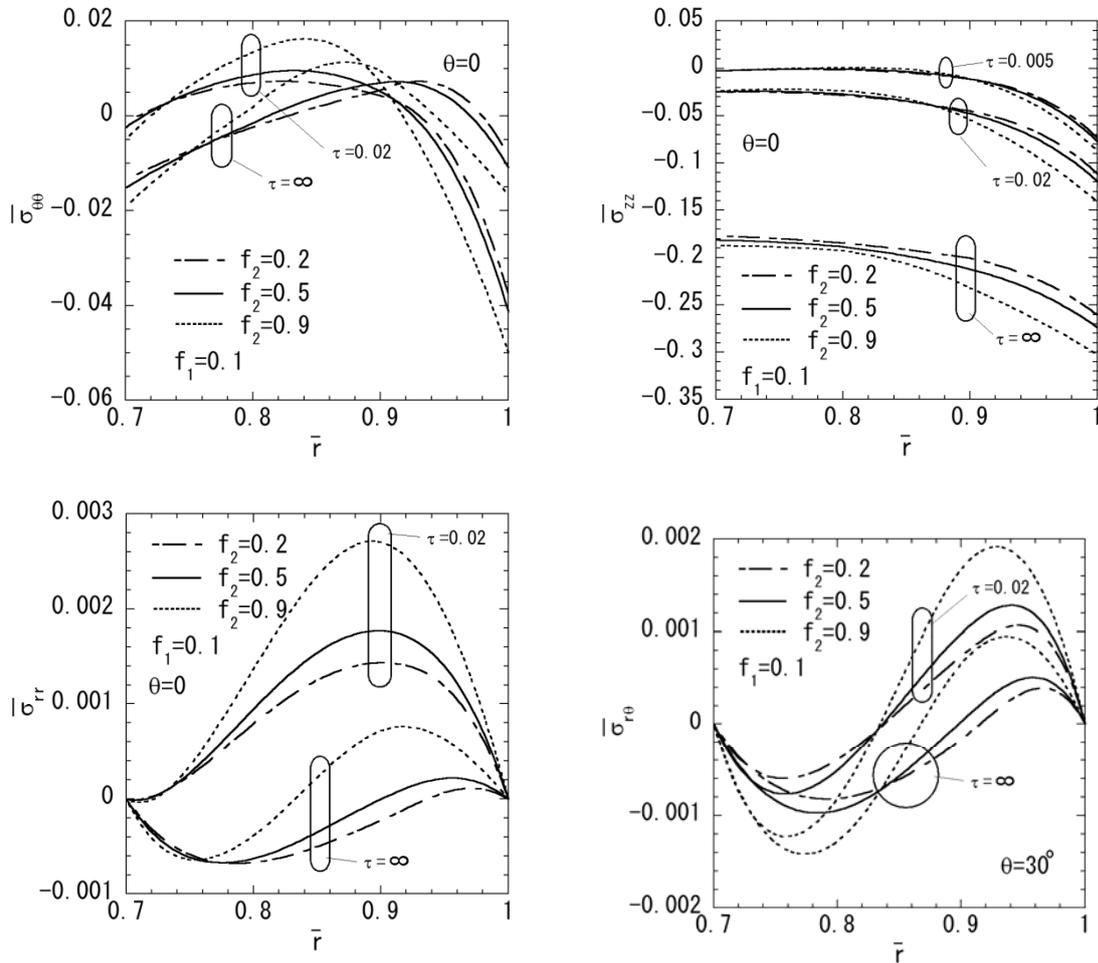
Fig. 8 Variation of thermal stresses in the radial direction (Material 3,  $N = 3$ ,  $\bar{r}_1 = 0.8$ ,  $\bar{r}_2 = 0.9$ ,  $f_1 = 0.1$ ): (a) normal stress  $\bar{\sigma}_{\theta\theta}$  ( $\theta = 0$ ), (b) normal stress  $\bar{\sigma}_{zz}$  ( $\theta = 0$ ), (c) normal stress  $\bar{\sigma}_{rr}$  ( $\theta = 0$ ), and (d) shearing stress  $\bar{\sigma}_{r\theta}$  ( $\theta = 30^\circ$ ).
