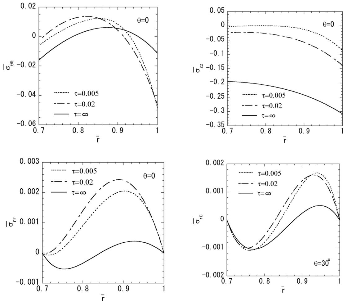
Fig. 9 Results for one-layered model (Material 4,  $N = 1$ ): (a) normal stress  $\bar{\sigma}_{\theta\theta}$  ( $\theta = 0$ ), (b) normal stress  $\bar{\sigma}_{zz}$  ( $\theta = 0$ ), (c) normal stress  $\bar{\sigma}_{rr}$  ( $\theta = 0$ ), and (d) shearing stress  $\bar{\sigma}_{r\theta}$  ( $\theta = 30^\circ$ )
