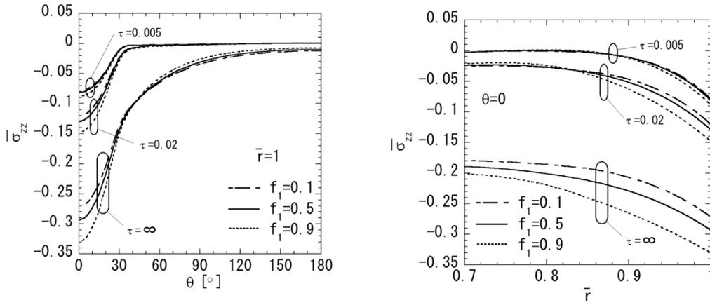
Fig. 3 Variation of thermal stress  $\bar{\sigma}_{zz}$  (Material 1,  $N = 2$ ,  $\bar{r}_1 = 0.85$ ): (a) variation in the heated surface ( $\bar{r} = 1.0$ ) and (b) variation in the radial direction ( $\theta = 0$ )
