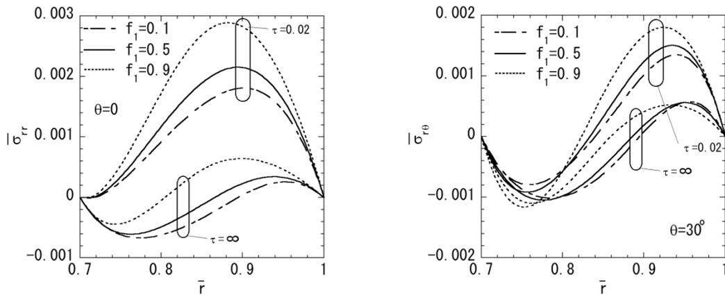
Fig. 4 Variation of thermal stresses in the radial direction (Material 1,  $N = 2$ ,  $\bar{r}_1 = 0.85$ ): (a) normal stress  $\bar{\sigma}_{rr}$  ( $\theta = 0$ ) and (b) shearing stress  $\bar{\sigma}_{r\theta}$  ( $\theta = 30^\circ$ )
